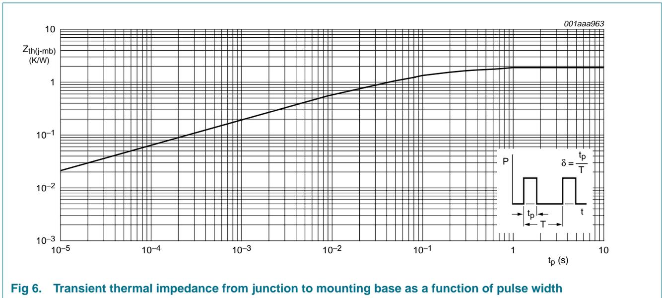
Fig 6. Transient thermal impedance from junction to mounting base as a function of pulse width
