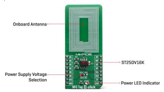
The ST25DV16K uses the I2C/SMBus compatible communication interface, offering a fast transfer mode (FTM), to achieve a fast link between RF and contact worlds, via a 256 byte buffer called Mailbox. This mailbox dynamic buffer of 256 byte can be filled or emptied via either RF or I2C.
