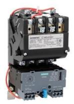
Non-reversing motor starter Size 1 Three phase full voltage Solid-state overload relay OLRelay amp range 5.5-22A 220-240/440-480VAC 60HZ coil Combination type No enclosure
