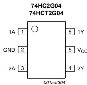
Figure 4. Pin configuration SOT363 and SOT457
