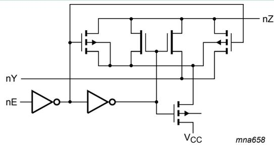
Fig. 3. Logic diagram (one switch)
