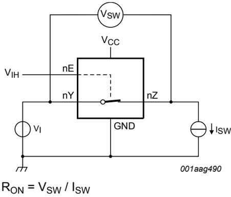
Fig. 9. Test circuit for measuring ON resistance
