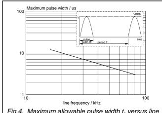
Fig.4. Maximum allowable pulse width  $t_{\rm p}$  versus line frequency; Basic horizontal deflection circuit.
