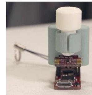
XMCT™ 2Go stacked with the TLV493D 3DSense Shield2Go and rotate knob
