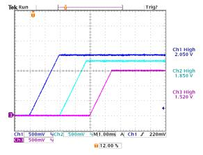
Figure 24. Turn-On with Different Rising Slew Rates. Rising Slew Rates are V1-1V/ms, V2-0.5V/ms, V3-0.2V/ms.
