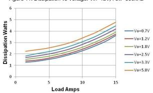
Figure 12 Dissipation vs Voltage. Vin=12V, Fsw=1MHz
