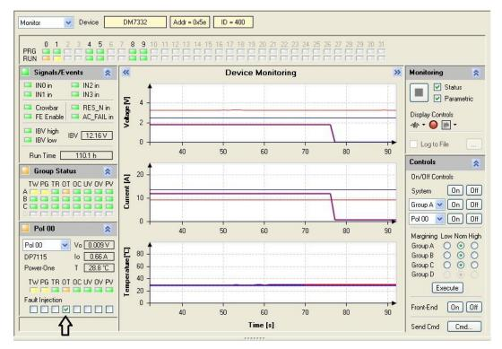
In Figure 55 we see the effects of injecting an Overtemp (OT) fault. Note that dPOL-0 shows an OT fault. dPOL-0 and -1 are in the same Group and fault propagation for the dPOL is to propagate to the group. dPOL -4 and above are in Groups B and C. Propagation is not enabled from Group A to B.
