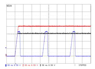
Figure 39 shows a scope capture an actual system when undervoltage error detection is set to not propagate.
