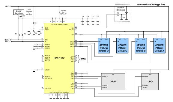
Shown in Figure 57 is a schematic of a typical application using at least one DP7115G point-of-load converter (dPOL). The system includes a DM7300 series Digital Power Manager (DPM), a DP7115G dPOL. Although only one dPOL is shown, other, additional dpwer® series dPOLs (Note SD and OK dashed lines "TO OTHER POLS") may be connected.
