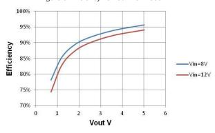
Figure 8 Efficiency vs Load. Vin=8V, Fsw=1MHz
