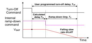
As it can be seen from the figure, the internally calculated delay  $T_{\text{D}}$  is determined by the equation below.
