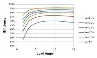
Figure 9 Efficiency vs Vout. Fsw=500KHz
