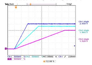
Figure 26 Two outputs delayed 5ms. All slew rates at 0.5V/ms
