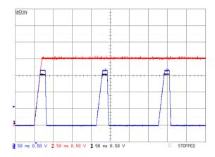
Since both Vo1 and Vo2 have the same delay and slew rate settings they will continue to turn off and on synchronously every 130ms, as shown in Figure 41, until the condition causing the undervoltage is removed.
