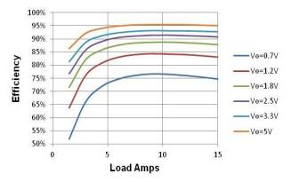
Figure 10 Efficiency vs Vout. Fsw=1MHz
