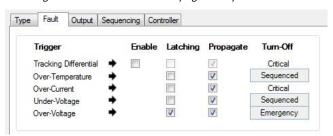
Figure 33. GUI dPOL Fault Propagation Option Window
