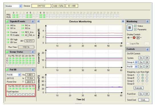
Figure 54. Fault Injection Controls In Monitor Window
