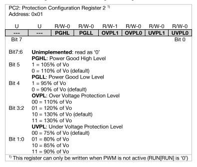
Note that the overvoltage and undervoltage protection thresholds and Power Good limits are defined as percentages of the output voltage. Therefore, the absolute levels of the thresholds change when the output voltage setpoint is changed either by output voltage adjustment or by margining.
