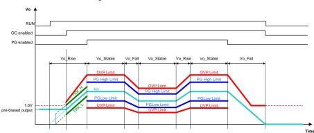
Figure 32. Protection Enable Conditions
