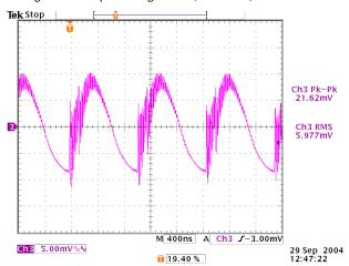
Figure 48. Output Voltage Noise, Full Load, 180° Interleave
