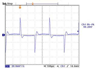
Figure 17 Transient response with non-zero Regulation.
