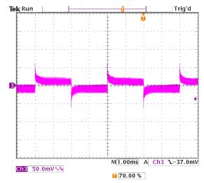
Increasing the Load Regulation parameter induces a droop, or offset, in the output at the higher current load.
