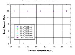
Figure 4. Available output current vs. ambient air temperature and airflow rates for converter DP7115G mounted horizontally with air flowing from input to output, MOSFET temperature 120°C, Vin = 12 V, Vout = 5 V, and Fsw= 1MHz
