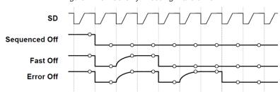
Figure 42. OK Severity Encoding Waveforms
