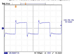
As the Load Regulation parameter is increased, step offsets in output voltage begin to appear, as shown in Figure 17 with non-zero Regulation.
