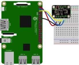
Pi 3V to sensor VCC (red wire)
