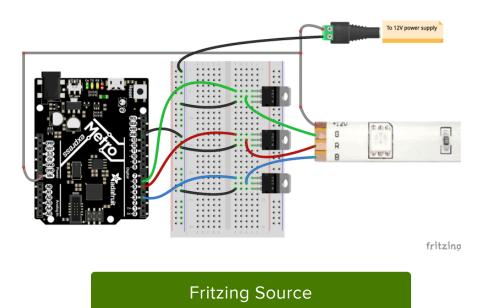
Note: Be sure to use PWM output pins from your board! Not all digital inputs/outputs support PWM output. Check your board's guide and pinout to confirm. Typically a
