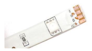
Melt some solder onto the pads to tin them and also burn away any left over rubber.
