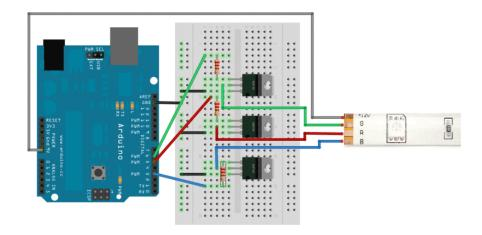
Connect a 9-12V power supply to the Arduino so that Vin supplies the high voltage to the LED strip. If you want, you can also just use a separate wire that connects to a power supply that provides about +12V. Make sure to connect the ground of that
