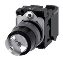
RONIS key-operated switch, 22 mm, round, plastic with metal front ring, lock number SB30, with 2 keys, 2 switch positions O-I, latching, actuating angle 90°, 10:30h/13:30h, key removal O+I, with holder, 1 NO, spring-type terminal, possible special locks: SB31, 421, 455, with laser labeling, upper case and lower case, always upper case at beginning of line
