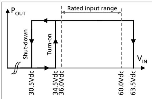
Fig. 3-2 Allowable output current below 36V input voltage
