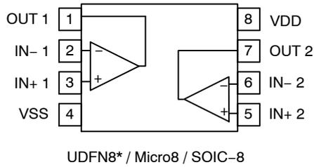
\*The exposed pad of the UDFN8 package can be floated or connected to VSS.
