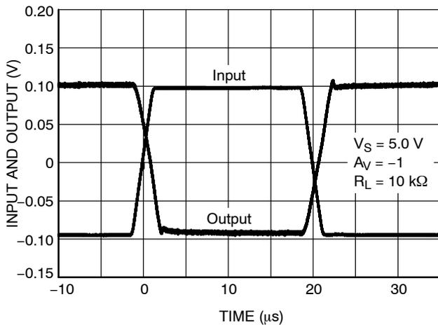
Figure 9. Small Signal Step Response
