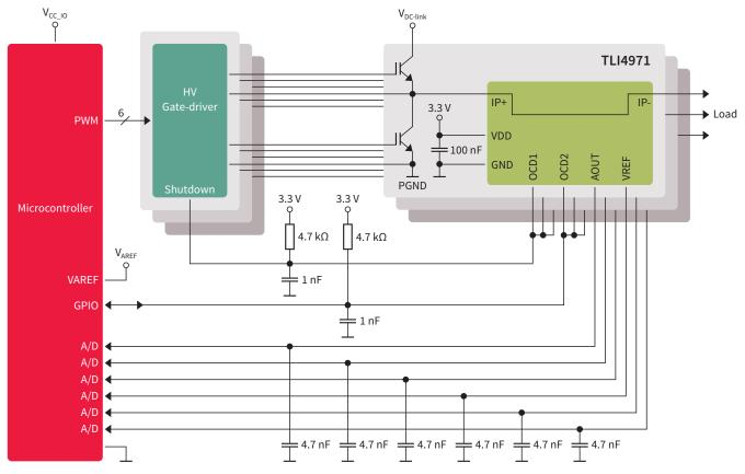
Application circuit for three phase system in differential configuration
