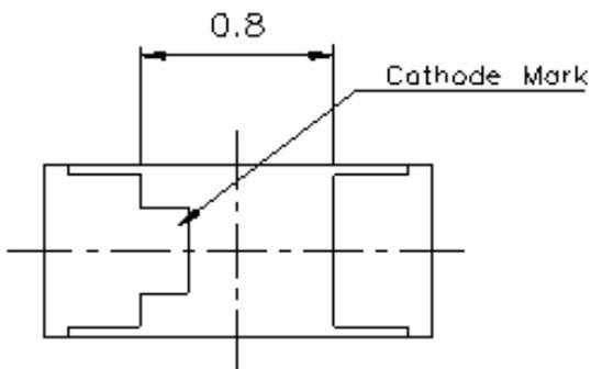
For reflow soldering (Propose)
