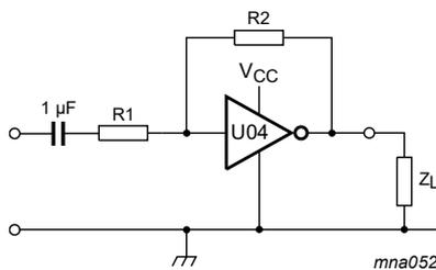
Maximum V<sub>o(p-p)</sub> = V<sub>CC</sub> - 1.5 V centered at 0.5 × V<sub>CC</sub>.
