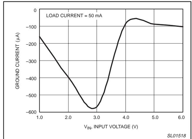
Figure 6. Ground current versus input voltage with load.
