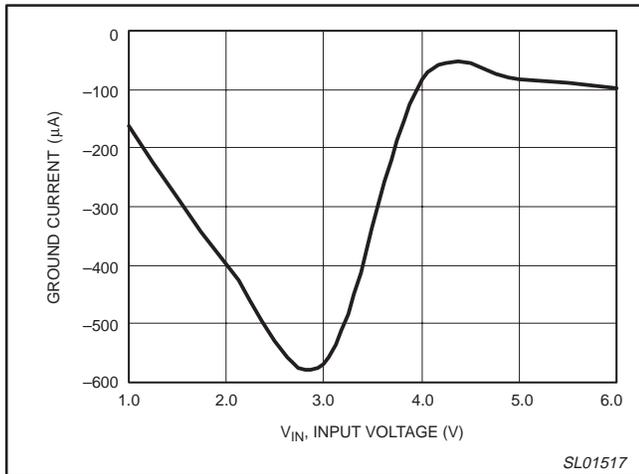
Figure 5. Ground current versus input voltage (no load).
