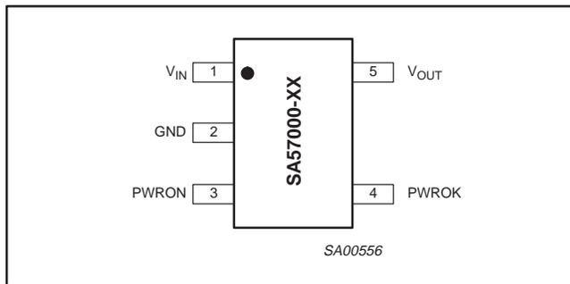
Figure 2. Pin configuration.
