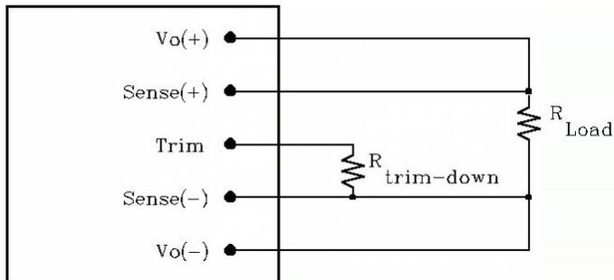
**Figure 17:** Circuit configuration for trim-down (decrease output voltage)
