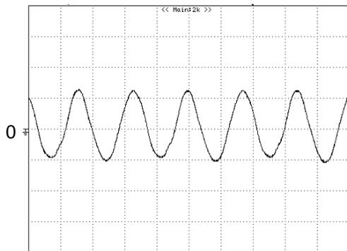
**Figure 14:** Output voltage ripple at nominal input voltage and rated load current ( $I_o$ =full load)(50 mV/div, 1 us/div)
