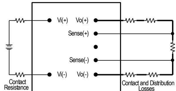
Figure 16: Effective circuit configuration for remote sense operation
