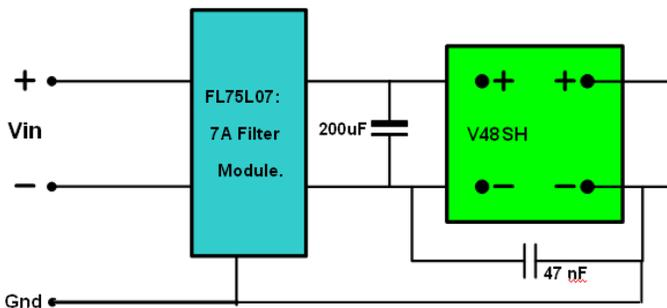
FL75L07 is Delta standard filter circuit module
