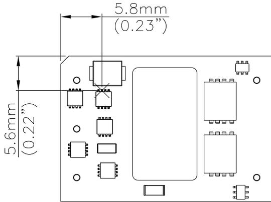
**Figure 20:** Temperature measurement location
