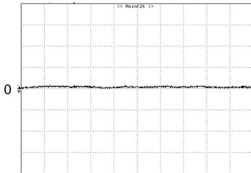
**Figure 12:** Input reflected ripple current,  $i_s$ , through a 12 μH source inductor at nominal input voltage and rated load current (20 mA/div, 1 us/div)
