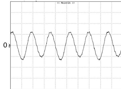
**Figure 11:** Input Terminal Ripple Current,  $i_c$ , at full rated output current and nominal input voltage with 12 μH source impedance and 33 μF electrolytic capacitor (100 mA/div, 1 us/div)
