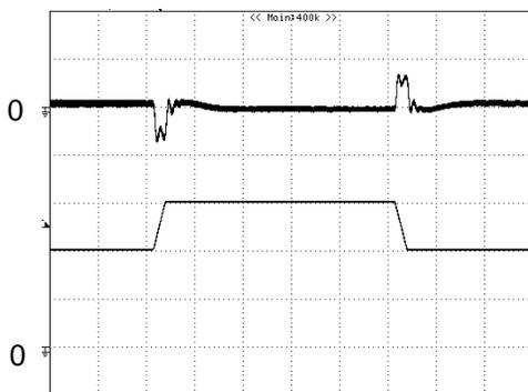
**Figure 8:** Output voltage response to step-change in load current (75%-50%-75% of  $I_{o, max}$ ;  $di/dt = 0.1A/\mu s$ ). Load cap: 10 $\mu F$  tantalum capacitor and 1 $\mu F$  ceramic capacitor. Top Trace:  $V_{out}$  (100mV/div, 200 $\mu s$ /div), Bottom Trace:  $I_{out}$  (5A/div). Scope measurement should be made using a BNC cable (length shorter than 20 inches). Position the load between 51 mm to 76 mm (2 inches to 3 inches) from the module
