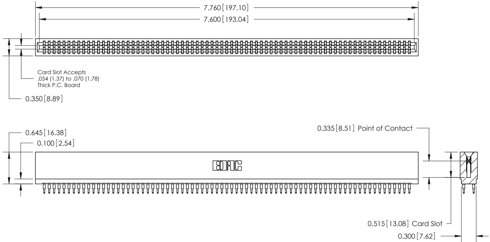
745 Series Ultra-Mate Card Edge Connector - Press Fit
