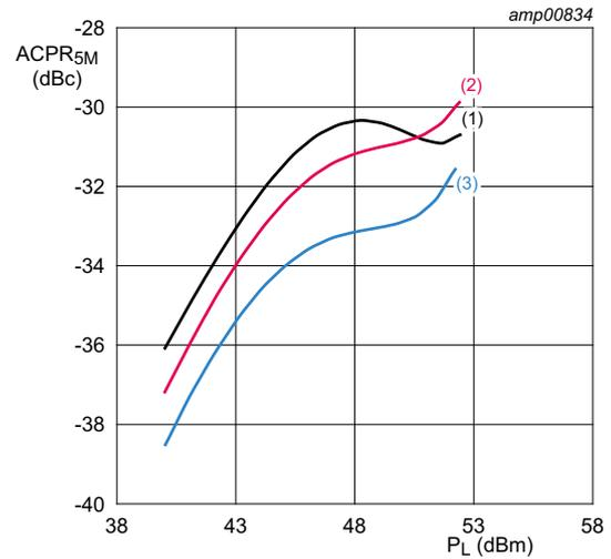
$V_{DS} = 32\text{ V}; I_{Dq} = 900\text{ mA}; V_{GS(amp)peak} = 1.2\text{ V}.$
