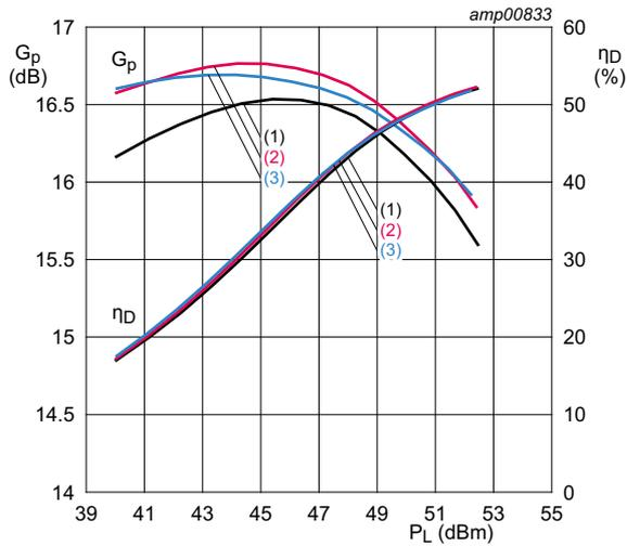
$V_{DS} = 32\text{ V}; I_{Dq} = 900\text{ mA}; V_{GS(amp)peak} = 1.2\text{ V}.$
