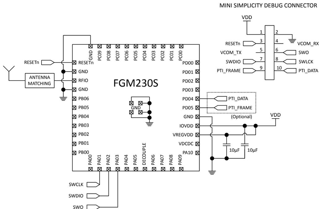
**Figure 5.1. Typical Connections for a Standalone Application**
