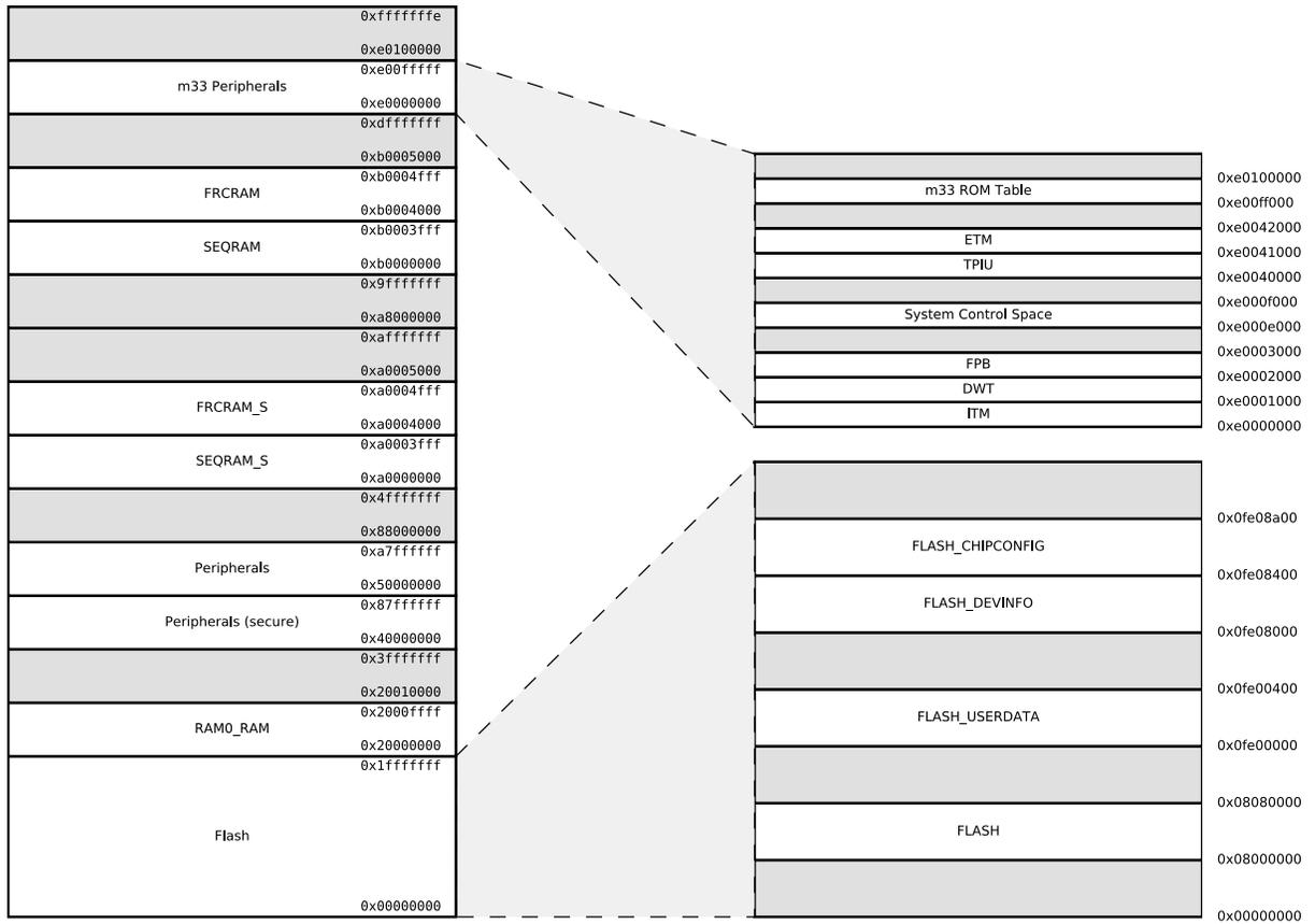
Figure 3.2. FGM230S Memory Map — Core Peripherals and Code Space
