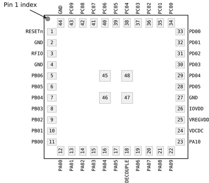
Figure 6.1. FGM230S Module Pinout
