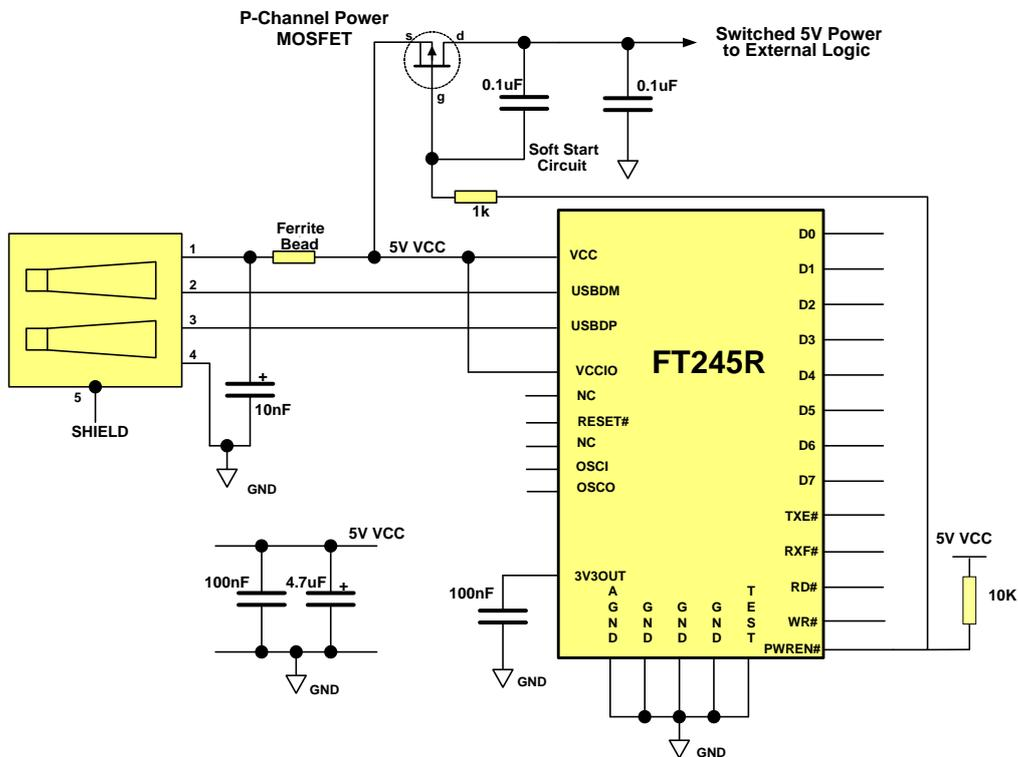
**Figure 6.3 Bus Powered with Power Switching Configuration**
