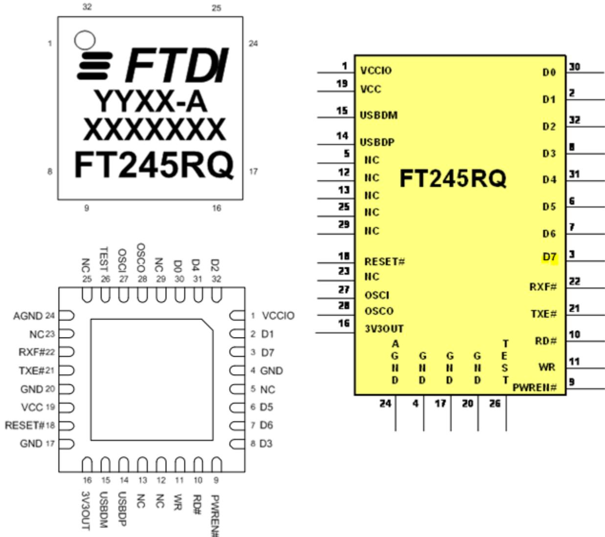
Figure 3.2 QFN-32 Package Pin Out and schematic symbol
