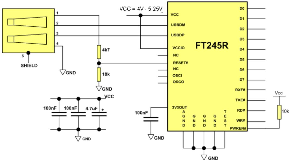
**Figure 6.2 Self-Powered Configuration**
