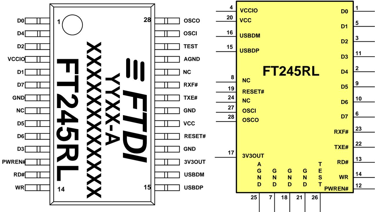
Figure 3.1 SSOP Package Pin Out and Schematic Symbol
