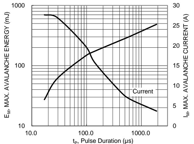
Figure 6. Single pulse Max. Avalanche Energy and Current
