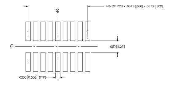
ALL DIMENSIONS ARE SYMMETRIC ABOUT THE CENTERLINE. STENCIL TO BE .0050[0.127] THICK
