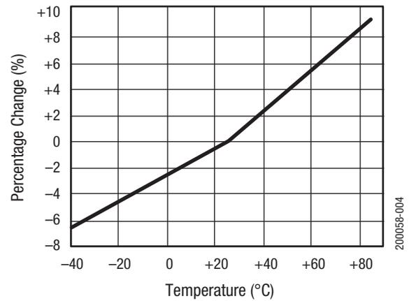
**Figure 4. Relative Series Resistance Change vs Temperature @ 500 MHz**
