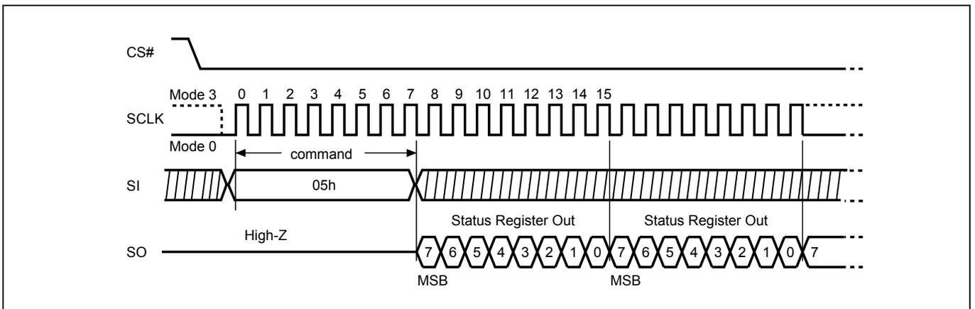
**Figure 24. Read Status Register (RDSR) Sequence (QPI Mode)**
