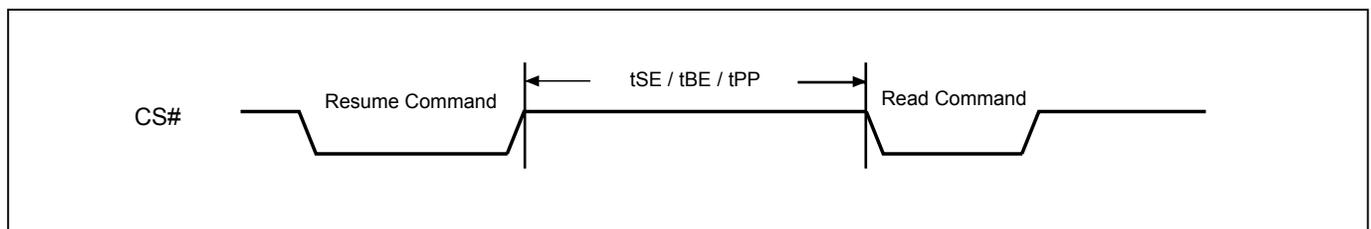
**Figure 98. Resume to Suspend Latency**
