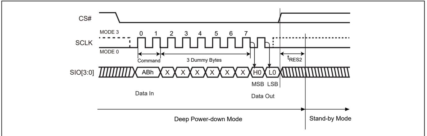
**Figure 20. Release from Deep Power-down (RDP) Sequence (SPI Mode)**
