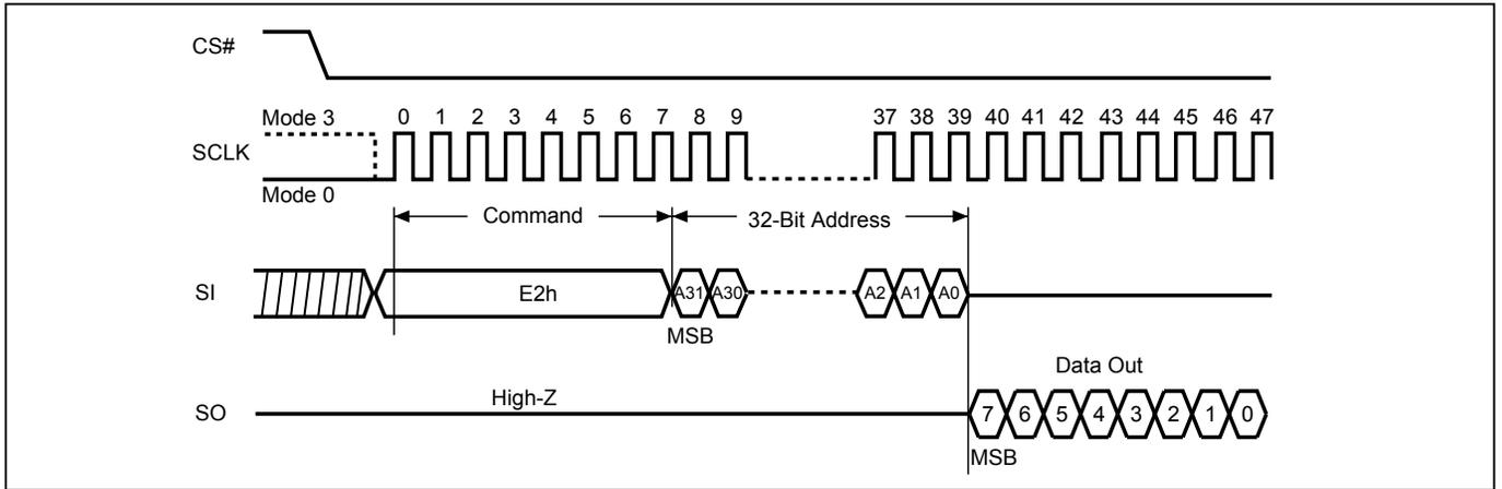
**Figure 89. SPB Erase (ESSPB) Sequence**
