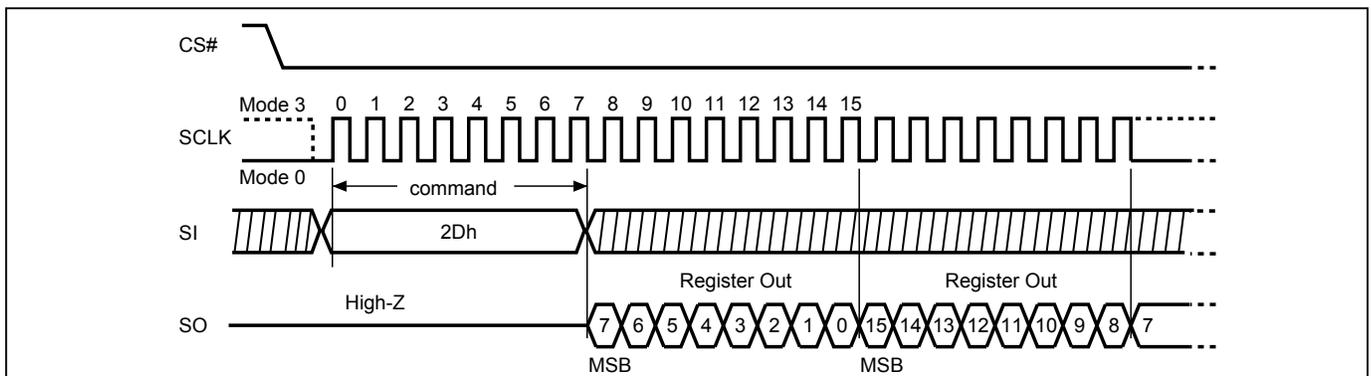
**Figure 87. Write Lock Register (WRLR) Sequence (SPI Mode)**
