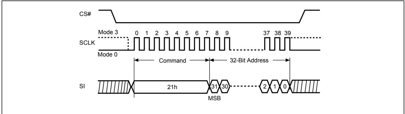
**Figure 56. Block Erase 32KB (BE32K4B) Sequence (SPI Mode)**
