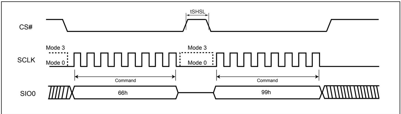
**Figure 101. Reset Sequence (QPI mode)**
