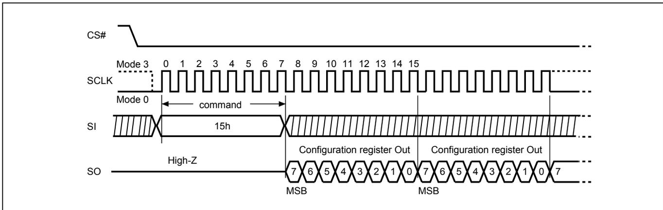
**Figure 26. Read Configuration Register (RDCR) Sequence (QPI Mode)**
