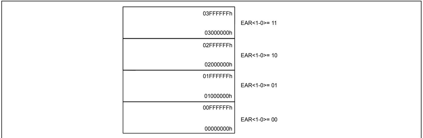
When under EAR mode, Read, Program, Erase operates in the selected segment by using 3-byte address mode.
