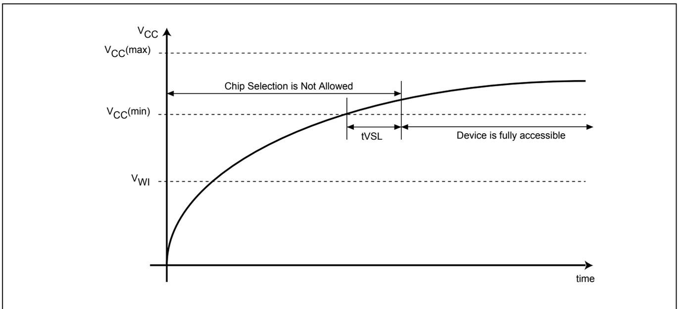
**Figure 112. Power Up/Down and Voltage Drop**
