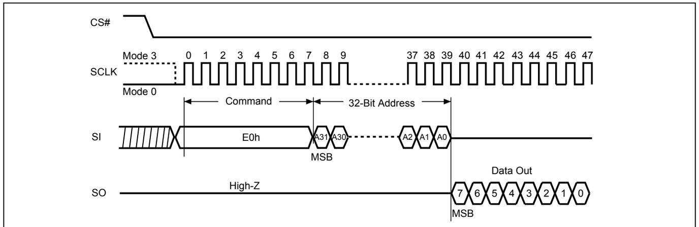
**Figure 92. Write DPB Register (WRDPB) Sequence**
