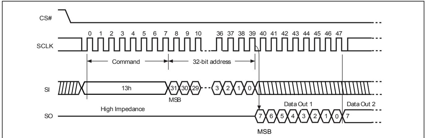
**Figure 50. Read Data Bytes at Higher Speed using 4 Byte Address Sequence (FASTREAD4B)**
