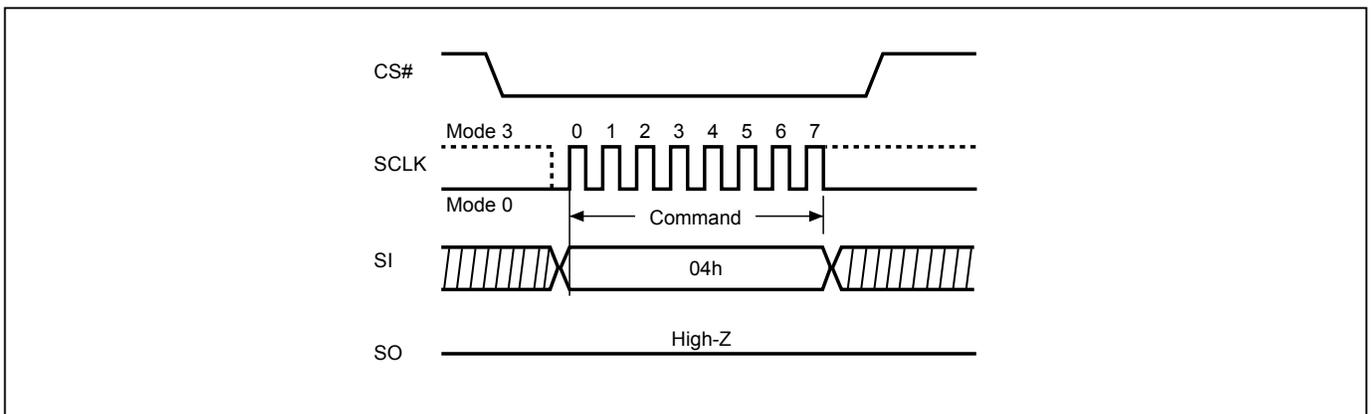
**Figure 16. Write Disable (WRDI) Sequence (QPI Mode)**
