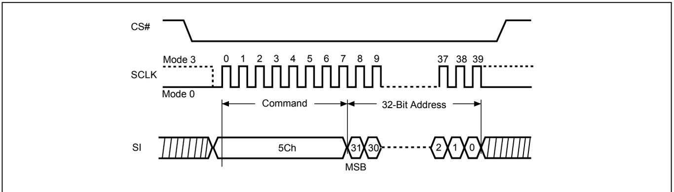
**Figure 57. Block Erase (BE4B) Sequence (SPI Mode)**
