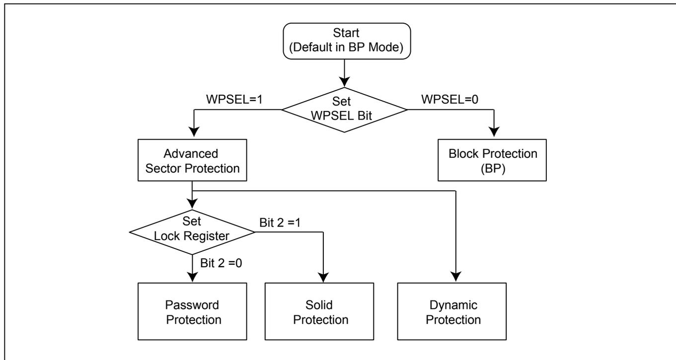
**Figure 84. WPSEL Flow**
