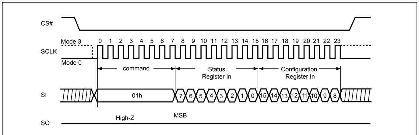
Note : The CS# must go high exactly at 8 bits or 16 bits data boundary to completed the write register command.
