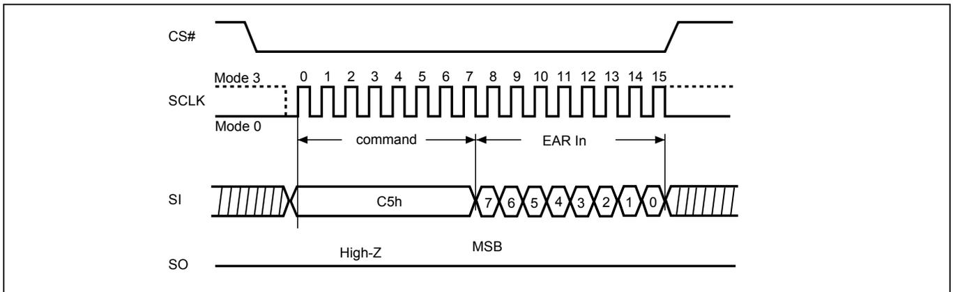
**Figure 8. Write EAR Register (WREAR) Sequence (QPI Mode)**
