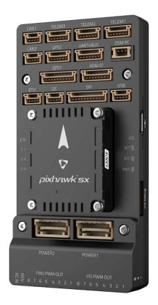
The Pixhawk® 5X is the latest update to the successful family of Pixhawk® flight controllers, based on the Pixhawk® FMUv5X Open Standard and the Pixhawk® Autopilot Bus Standard.
