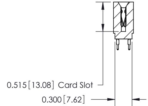
745 Series Ultra-Mate Card Edge Connector - Press Fit
