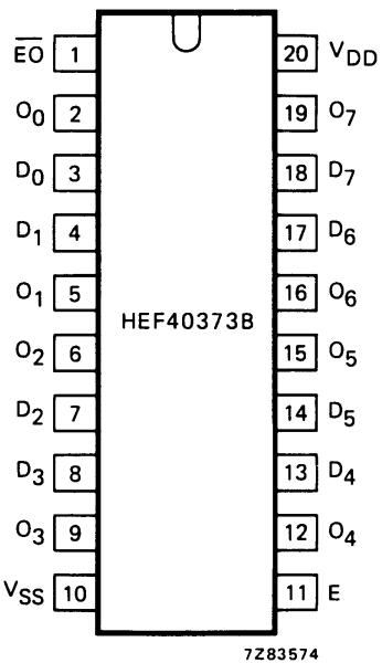
Fig.2 Pinning diagram.
