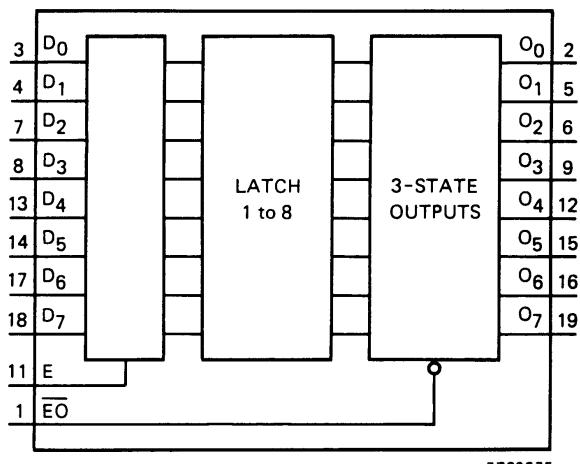
Fig.1 Functional diagram.
