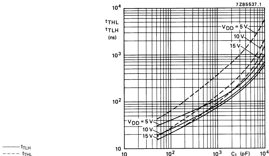
Fig.7 Output transition times as a function of the load capacitance. .
