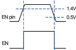
Figure 3. Enable Threshold Schematic and Timing Sequence
