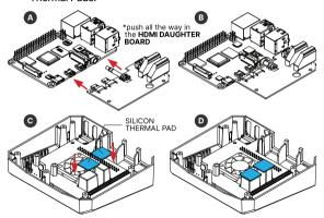
Carefully connect Raspberry Pi GPIO to Power and Cooling Board. Press POWER ON button to start.
