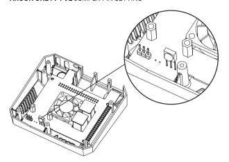
Use longer round head screws to fasten bottom cover and place rubber footings.
