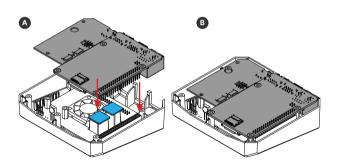
Use shorter flat head screws to fasten Raspberry Pi and HDMI Board assembly to top case.
