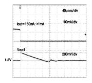
Fig.42. Load Response (VOUT1=1.2V) IOUT=150mA→1mA
