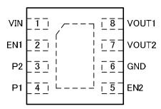
Note : Recommend connecting the Thermal Pad to the GND for excellent power dissipation.
