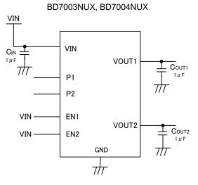
Figure2. Application Circuit
