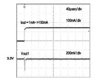
Fig.41. Load Response (VOUT1=3.3V) IOUT=1mA→150mA
