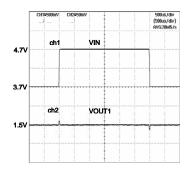
Fig.36. VIN Response (VOUT1=1.5V) IOUT=50mA
