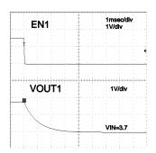
Fig.33. Discharge Time (VOUT1=1.8V) IOUT=0mA
