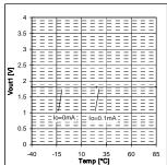
Fig.18. VOUT - Temp (VOUT1=1.8V)
