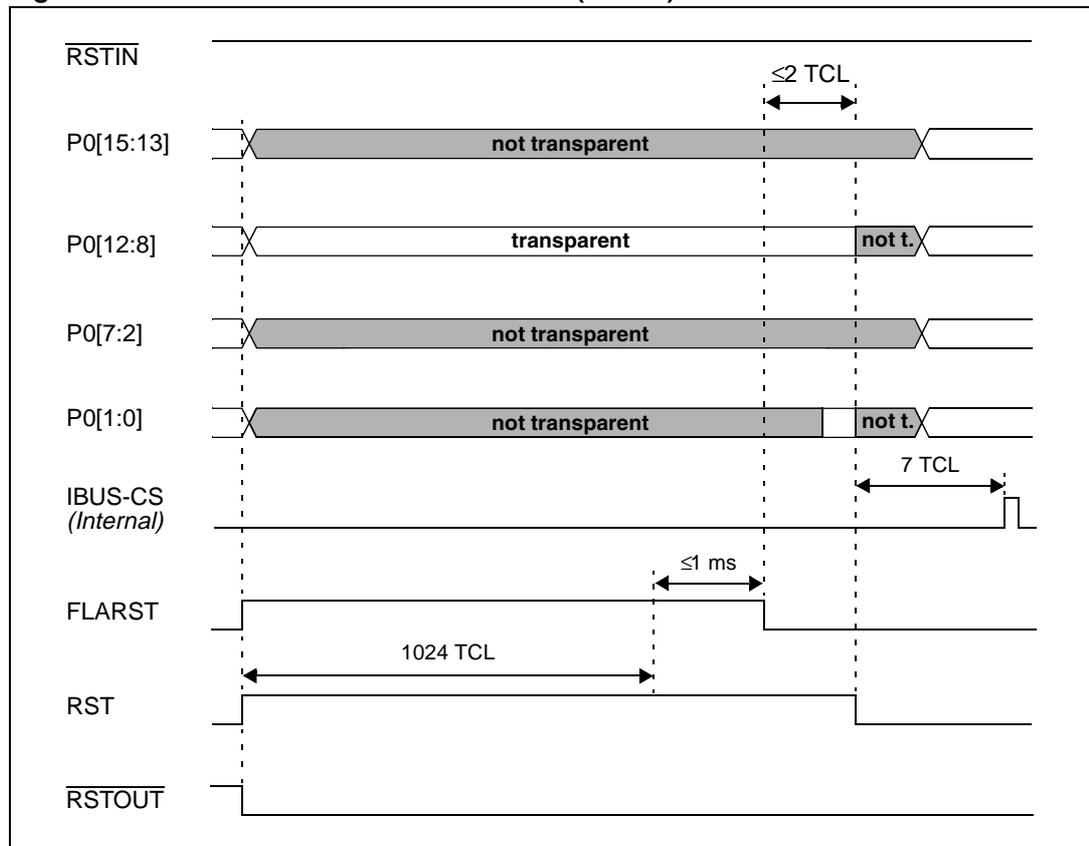
Figure 24. SW / WDT unidirectional RESET ( $\overline{EA} = 0$ )
