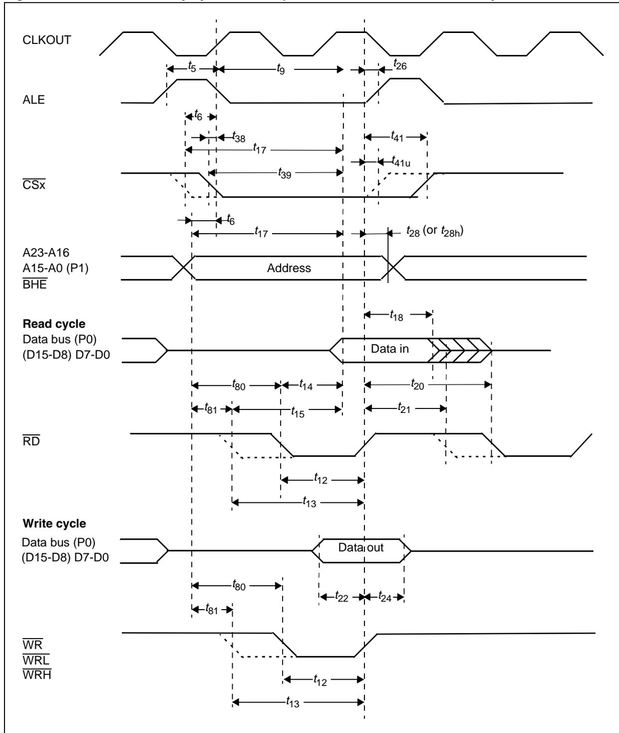
Figure 53. External memory cycle: Demultiplexed bus, with/without r/w delay, extended ALE
