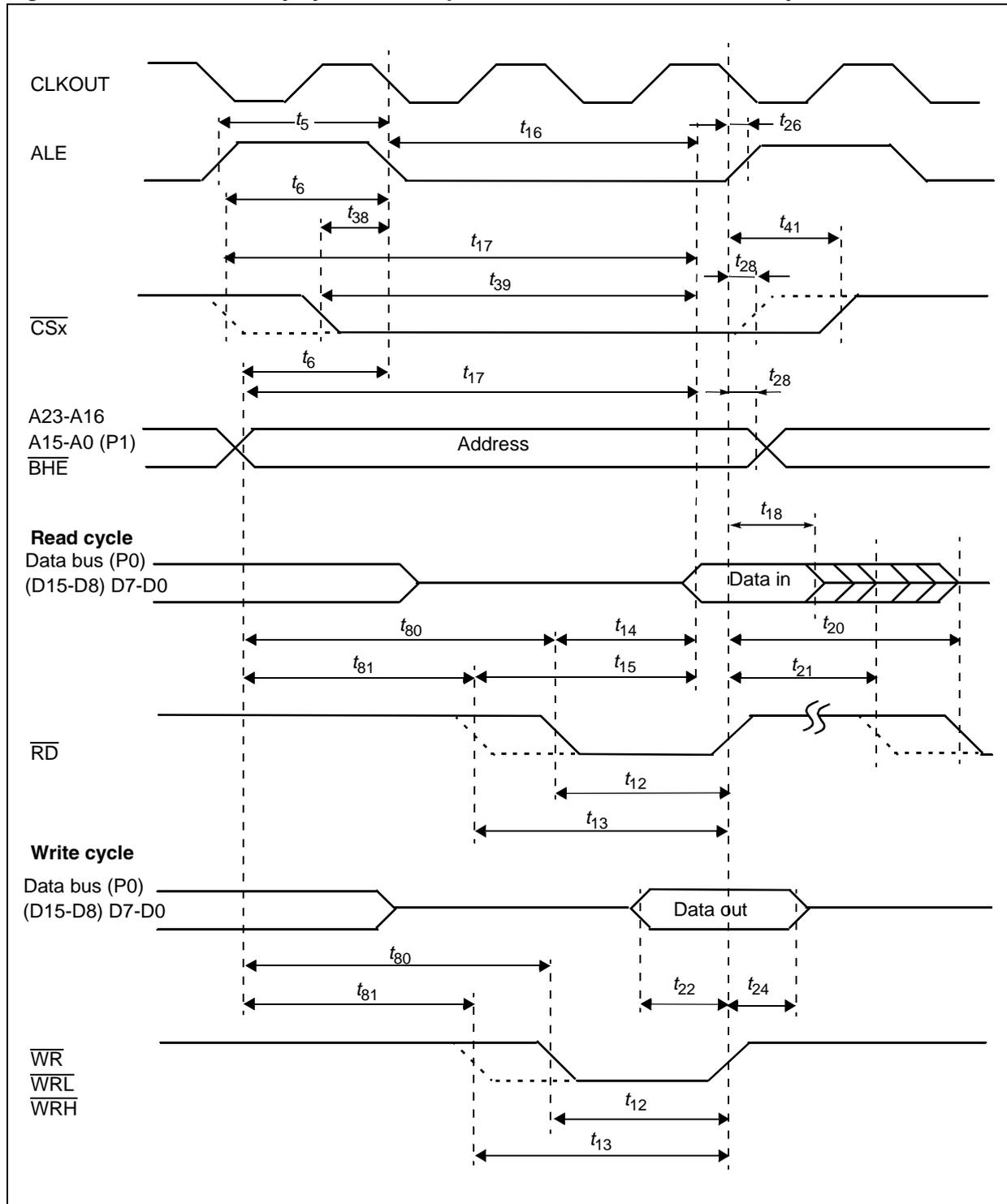
Figure 54. External memory cycle: Demultipl. bus, with/without r/w delay, normal ALE, r/w CS
