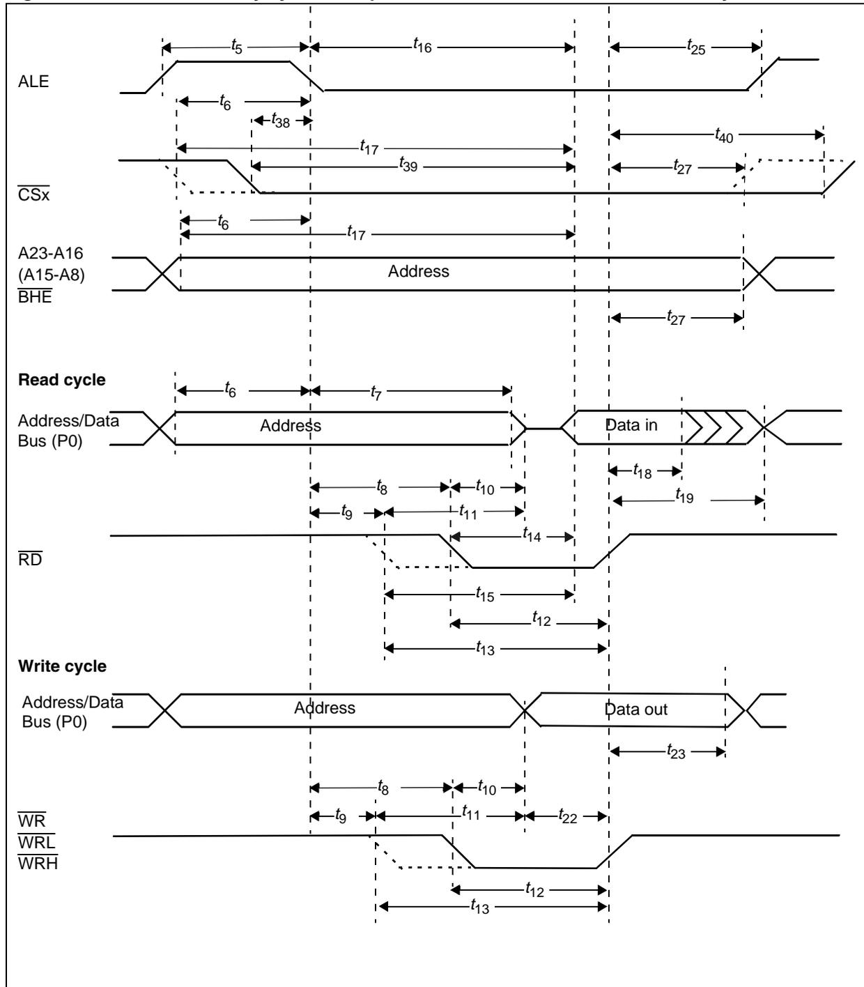
Figure 50. External memory cycle: Multiplexed bus, with/without r/w delay, normal ALE, r/w CS
