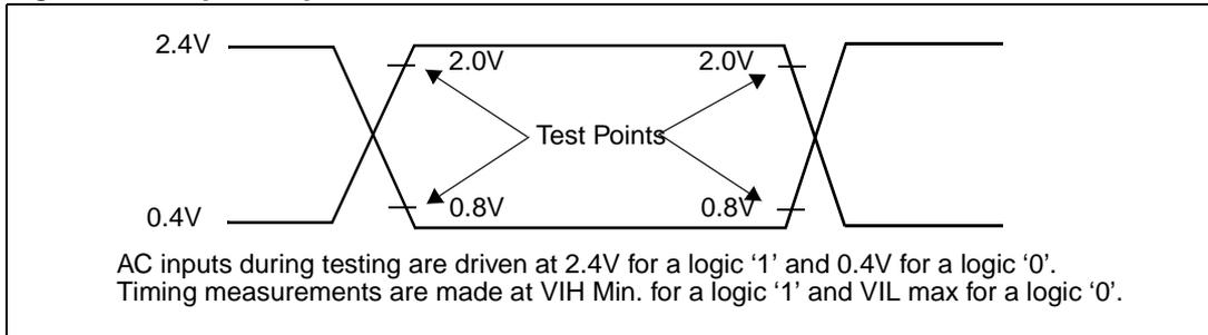
Figure 42. Float waveform
