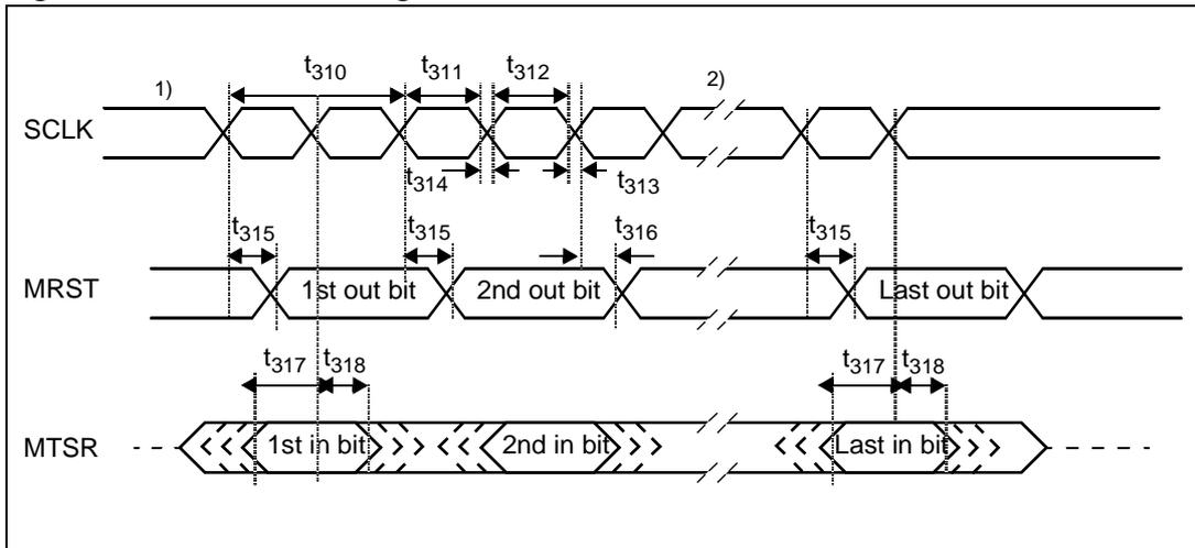
1. The phase and polarity of shift and latch edge of SCLK is programmable. This figure uses the leading clock edge as shift edge (drawn in bold), with latch on trailing edge (SSCPH = 0b), Idle clock line is low, leading clock edge is low-to-high transition (SSCPO = 0b).
