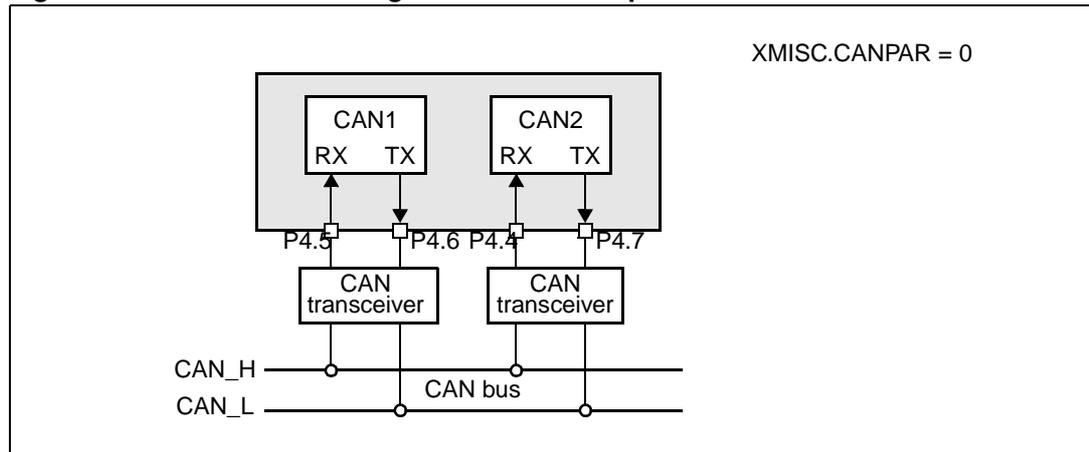
The ST10F273E also supports single CAN Bus multiple (dual) interfaces using the open drain option of the CANx\_TxD output as shown in [Figure 12](#). Thanks to the OR-Wired Connection, only one transceiver is required. In this case the design of the application must take in account the wire length and the noise environment.
