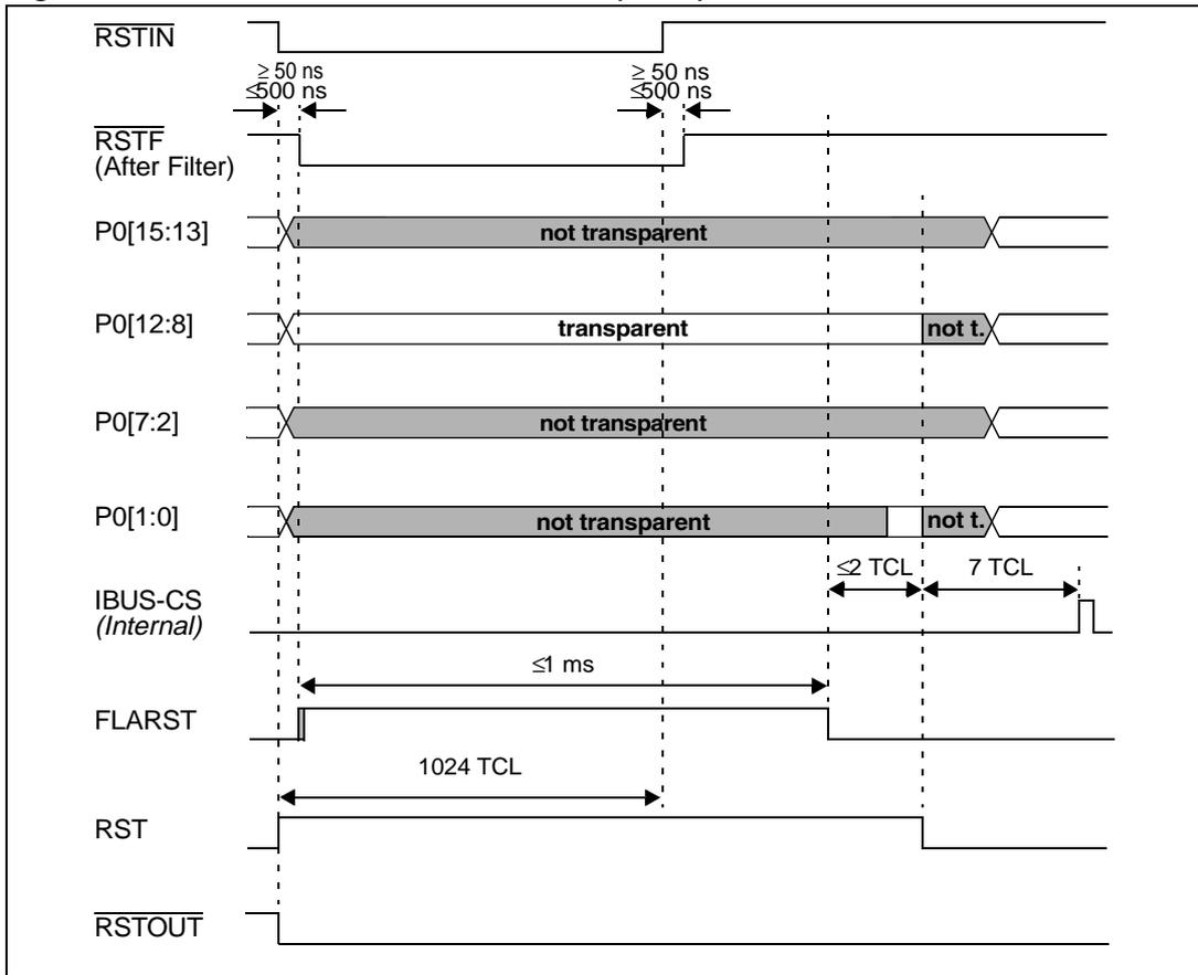
Figure 26. SW / WDT bidirectional RESET ( $\overline{EA} = 0$ )
