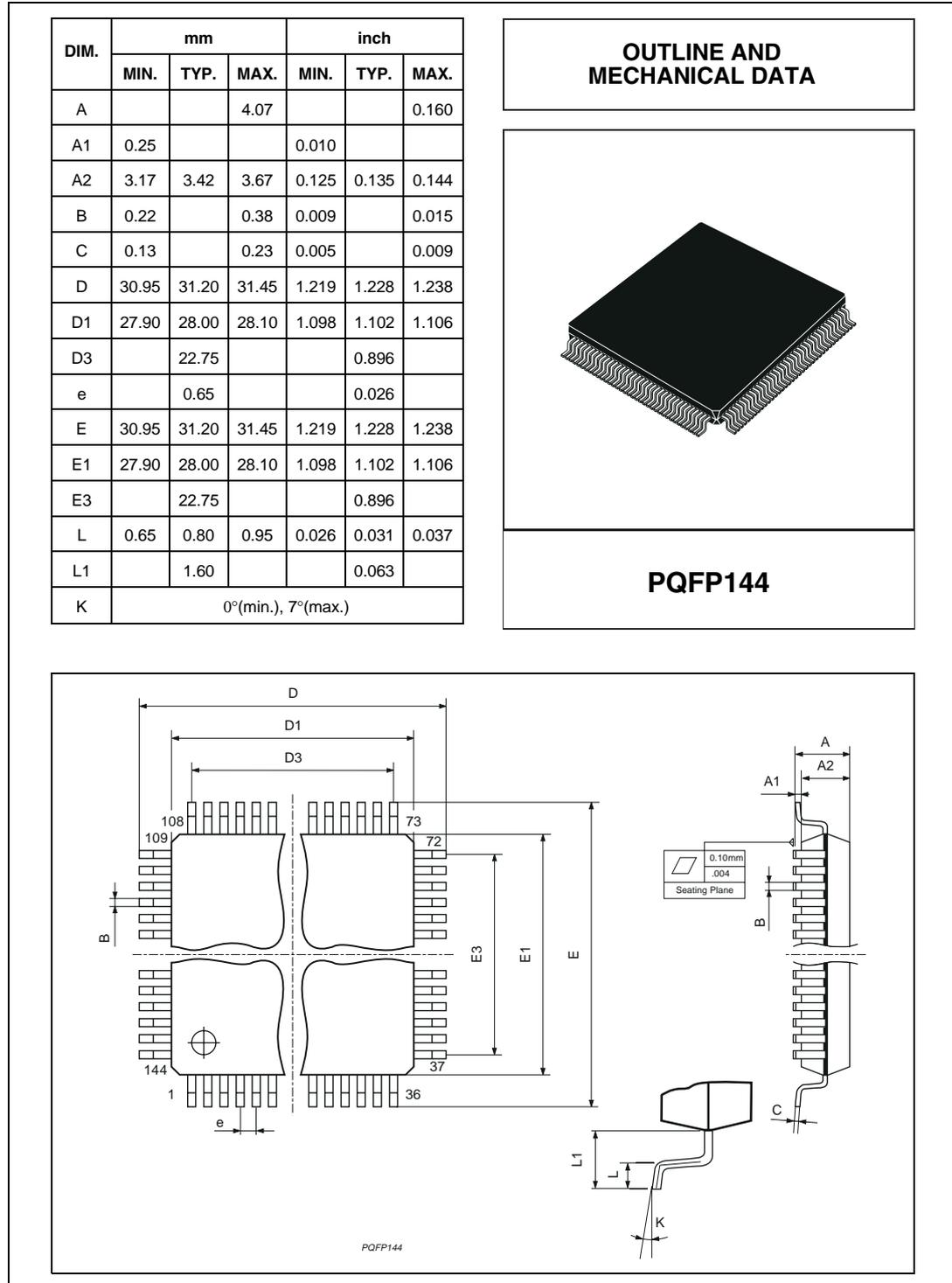
Figure 62. TQFP144 mechanical data and package dimension
