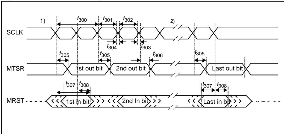
1. The phase and polarity of shift and latch edge of SCLK is programmable. This figure uses the leading clock edge as shift edge (drawn in bold), with latch on trailing edge (SSCPH = 0b), Idle clock line is low, leading clock edge is low-to-high transition (SSCPO = 0b).
