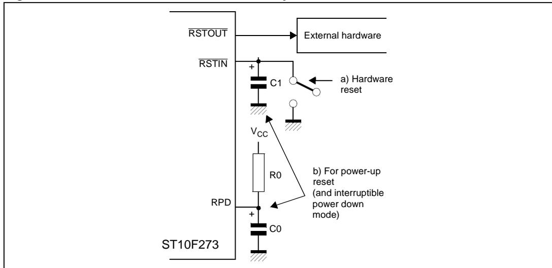
The minimum reset circuit of [Figure 28](#) is not adequate when the  $\overline{RSTIN}$  pin is driven from the ST10F273E itself during software or watchdog triggered resets, because of the capacitor C1 that will keep the voltage on  $\overline{RSTIN}$  pin above  $V_{IL}$  after the end of the internal reset sequence, and thus will trigger an asynchronous reset sequence.
