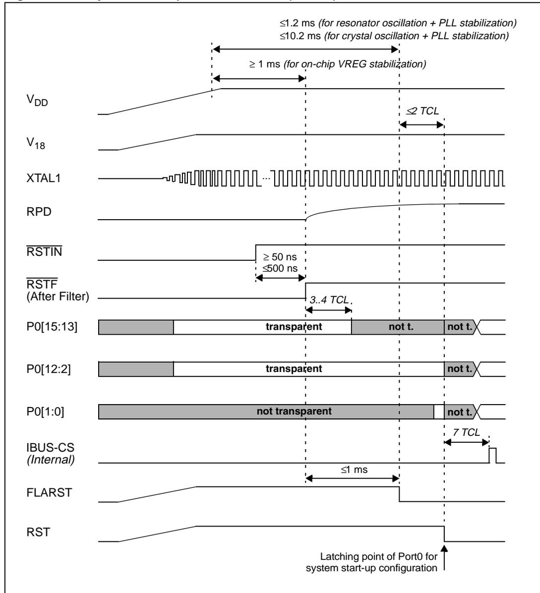
Figure 16. Asynchronous power-on RESET ( $\overline{EA} = 0$ )
