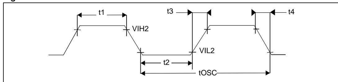
*Note:* When Direct Drive is selected, an external clock source can be used to drive XTAL1. The maximum frequency of the external clock source depends on the duty cycle: when 64 MHz is used, 50% duty cycle shall be granted (low phase = high phase = 7.8ns); when for instance 32 MHz is used, a 25% duty cycle can be accepted (minimum phase, high or low, again equal to 7.8ns).
