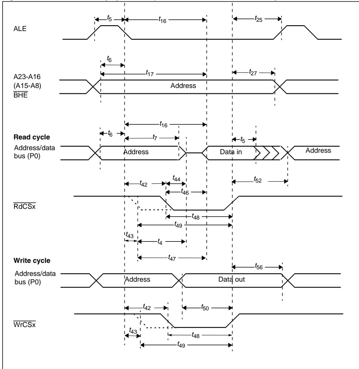
Figure 51. External memory cycle: Multiplexed bus, with/without r/w delay, extended ALE, r/w CS
