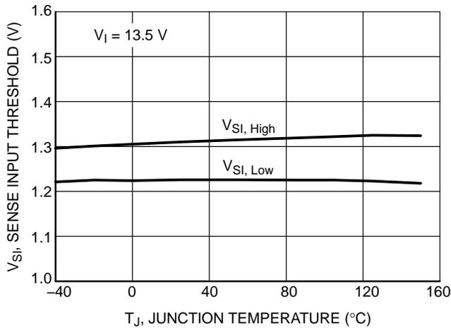
Figure 11. Sense Threshold  $V_{Sl}$  vs. Temperature  $T_J$
