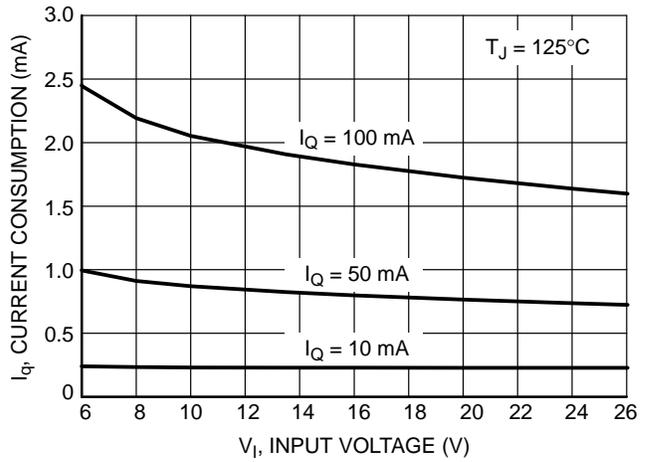
Figure 16. Quiescent Current  $I_q$  vs. Input Voltage  $V_I$
