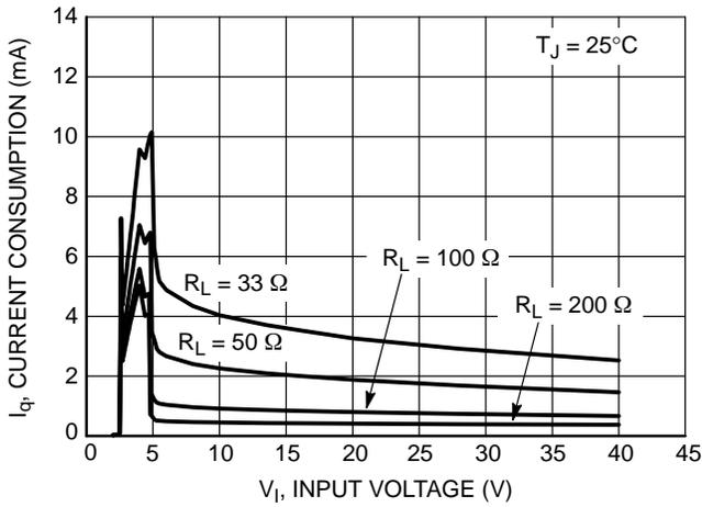
Figure 9. Current Consumption  $I_q$  vs. Input Voltage  $V_I$
