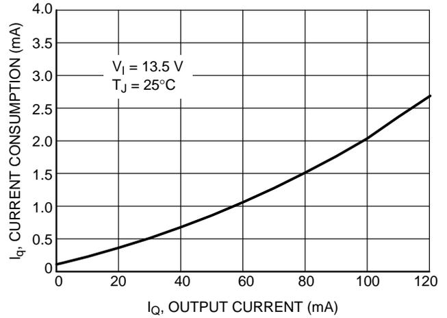
Figure 14. Current Consumption  $I_q$  vs. Output Current  $I_Q$
