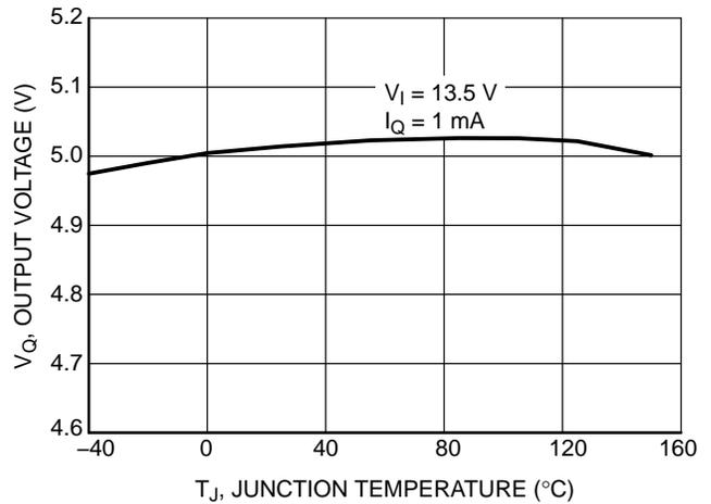
Figure 12. Output Voltage  $V_Q$  vs. Temperature  $T_J$
