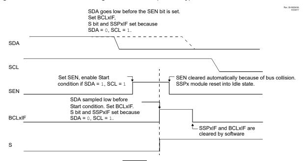
Figure 35-33. Bus Collision During Start Condition (SDA Only)
