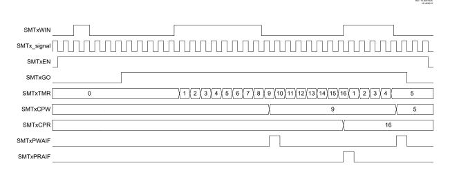
Figure 37-21. Windowed Counter Mode, Single Acquisition Timing Diagram
