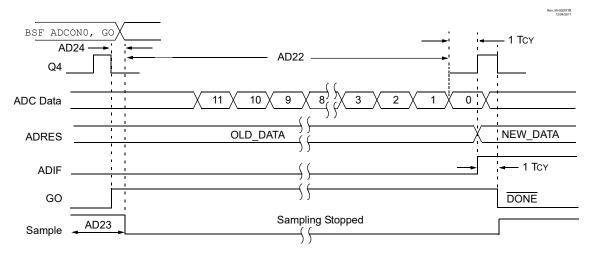
Figure 42-11. ADC Conversion Timing (ADC Clock from ADCRC)
