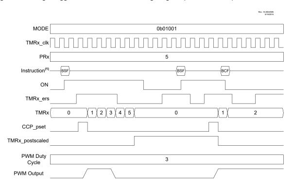
Figure 27-8. Edge-Triggered One-Shot Mode Timing Diagram (MODE = 01001)
