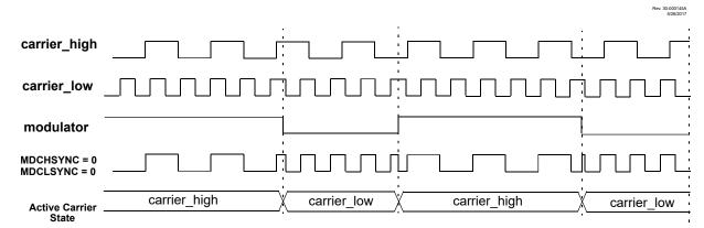
Figure 32-4. Carrier High Synchronization (MDCHSYNC = 1, MDCLSYNC = 0)
