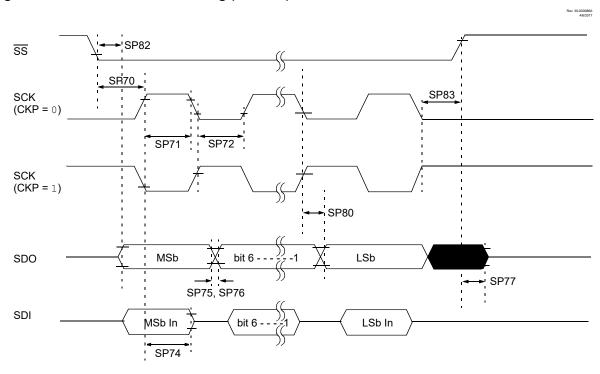
Figure 42-20. SPI Slave Mode Timing (CKE = 1)
