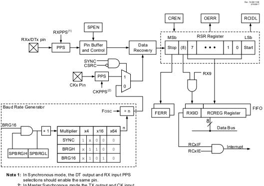
Figure 36-2. EUSART Receive Block Diagram
