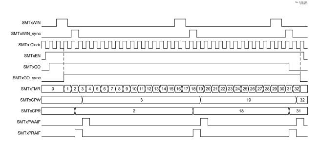
Figure 37-16. Capture Mode, Single Acquisition Timing Diagram
