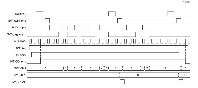
Figure 37-12. Gated Windowed Measurement Mode, Single Acquisition Timing Diagram
