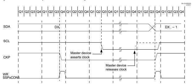
Figure 35-23. Clock Synchronization Timing
