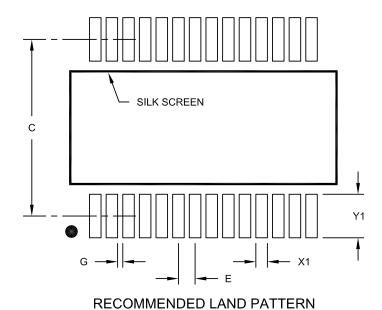
MILLIMETERS Units Dimension Limits MIN NOM MAX 0.65 BSC Contact Pitch Ε Contact Pad Spacing С 7.20 Contact Pad Width (X28) 0.45 X1 Contact Pad Length (X28) Y1 1.75 Distance Between Pads G 0.20
