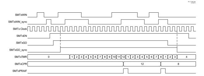
Figure 37-10. Windowed Measurement Mode, Single Acquisition Timing Diagram
