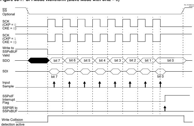
Figure 35-7. SPI Mode Waveform (Slave Mode with CKE = 0)
