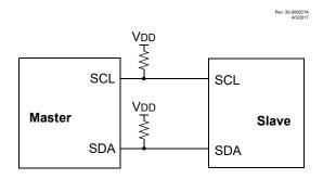
The I<sup>2</sup>C bus can operate with one or more master devices and one or more slave devices.
