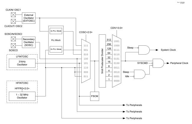
Figure 9-1. Simplified PIC® MCU Clock Source Block Diagram
