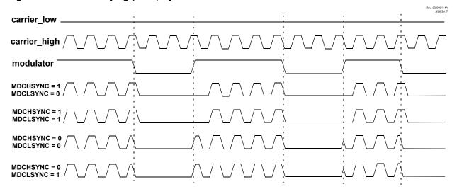
Figure 32-3. No Synchronization (MDCHSYNC = 0, MDCLSYNC = 0)
