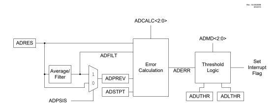
The operation of the ADC computational features is controlled by MD bits.
