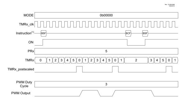
1. BSF and BCF represent Bit-Set File and Bit-Clear File instructions executed by the CPU to set or clear the ON bit of TxCON. CPU execution is asynchronous to the timer clock input.
