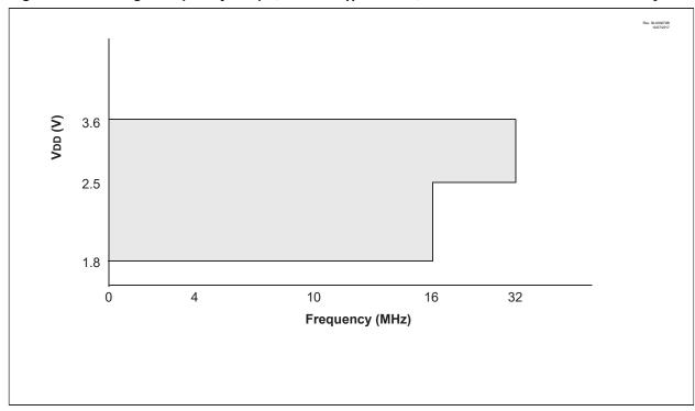
Figure 42-2. Voltage Frequency Graph, -40°C ≤ T<sub>A</sub>≤ +125°C, for PIC16LF18455/56 Devices only
