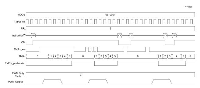
Figure 27-11. Rising Edge-Triggered Monostable Mode Timing Diagram (MODE = 10001)
