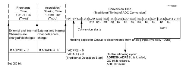
For correct conversion, the appropriate T<sub>AD</sub> specification must be met. Access the "ADC Timing Specifications" link at the end of this topic for more information. The following table below gives examples of appropriate ADC clock selections.
