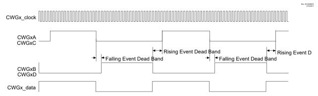
Note: CWGx\_rising\_src = CCP1\_out, CWGx\_falling\_src = ~CCP1\_out
