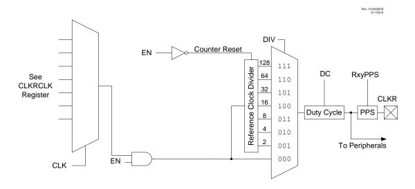
Figure 34-2. Clock Reference Timing
