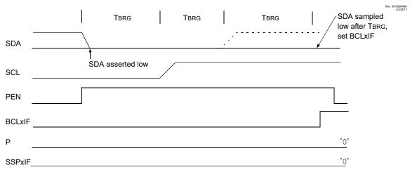
Figure 35-39. Bus Collision During a Stop Condition (Case 2)
