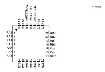
Note: It is recommended that the exposed bottom pad be connected to V<sub>SS</sub>.
