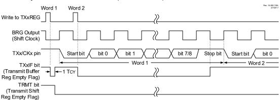
Figure 36-4. Asynchronous Transmission (Back-to-Back)
