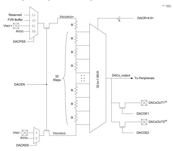
Figure 21-1. Digital-to-Analog Converter Block Diagram
