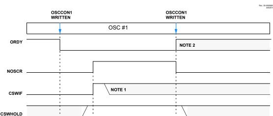
Figure 9-8. Clock Switch Abandoned
