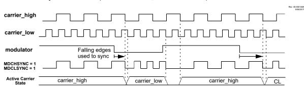
Figure 32-6. Full Synchronization (MDCHSYNC = 1, MDCLSYNC = 1)
