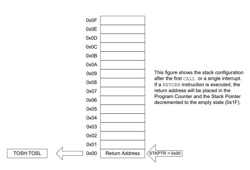
Figure 7-6. Accessing the Stack Example 3
