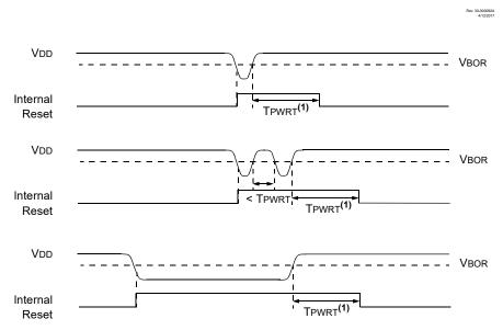
**Note:** T<sub>PWRT</sub> delay only if PWRTS bit field is programmed to a value different from '11'.
