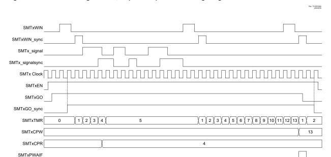
Figure 37-13. Time of Flight Mode, Repeat Acquisition Timing Diagram
