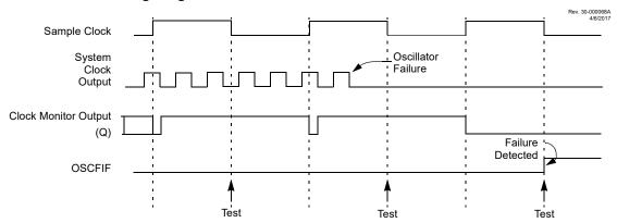
**Note:** The system clock is normally at a much higher frequency than the sample clock. The relative frequencies in this example have been chosen for clarity.
