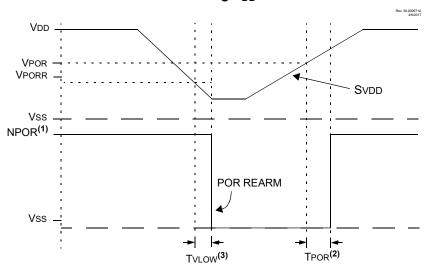
Figure 42-3. POR and POR Rearm with Slow Rising  $V_{DD}$
