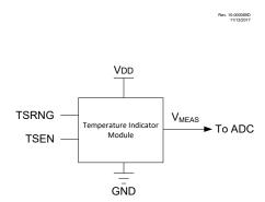
The output of the circuit is measured using the internal Analog-to-Digital Converter. A channel is reserved for the temperature circuit output. Refer to the ADC link below for detailed information.
