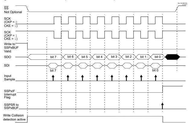
Figure 35-8. SPI Mode Waveform (Slave Mode with CKE = 1)
