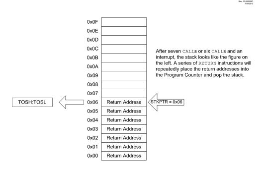
Figure 7-7. Accessing the Stack Example 4
