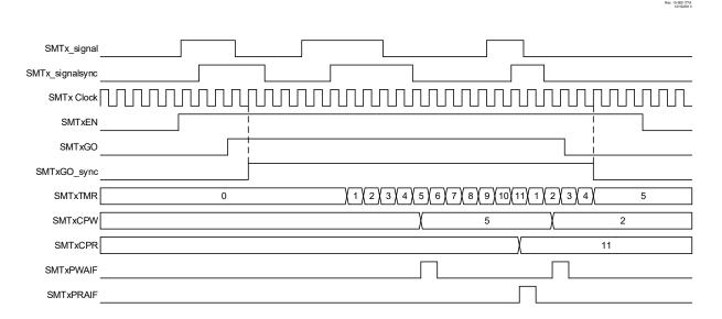
Figure 37-6. Period and Duty-Cycle, Single Acquisition Mode Timing Diagram
