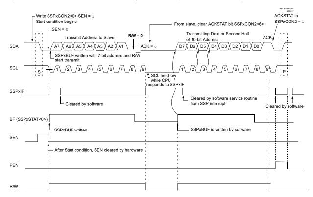
Figure 35-28. I<sup>2</sup>C Master Mode Waveform (Transmission, 7 or 10-bit Address)
