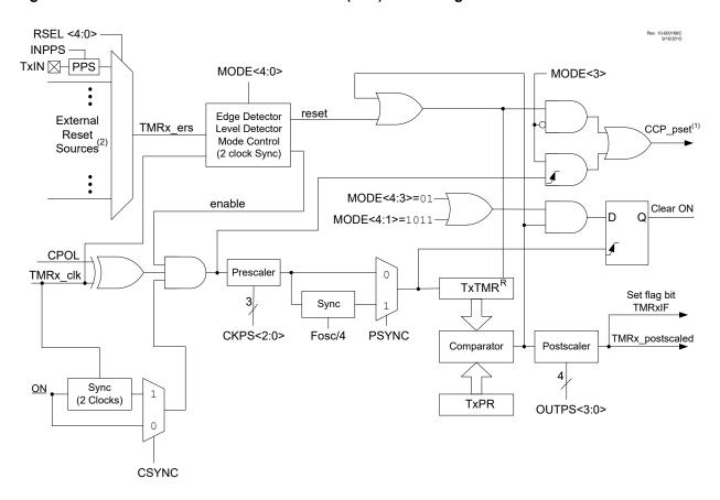
Figure 27-1. Timer2 with Hardware Limit Timer (HLT) Block Diagram
