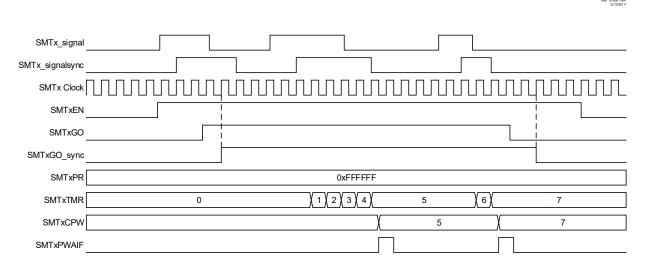
Figure 37-4. Gated Timer Mode, Single Acquisition Timing Diagram
