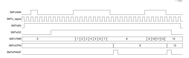
Figure 37-19. Gated Counter Mode, Single Acquisition Timing Diagram
