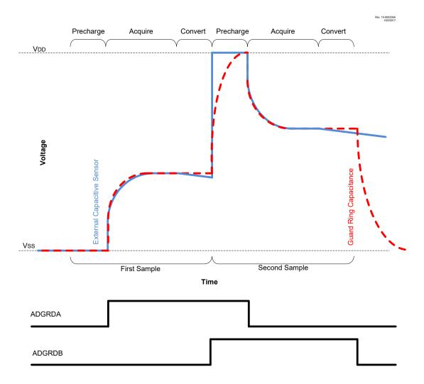
Figure 20-8. Differential CVD with Guard Ring Output Waveform
