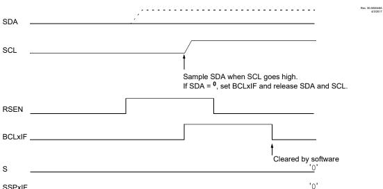
Figure 35-36. Bus Collision During a Repeated Start Condition (Case 1)
