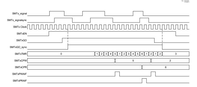
Figure 37-8. High and Low Measurement Mode, Single Acquisition Timing Diagram
