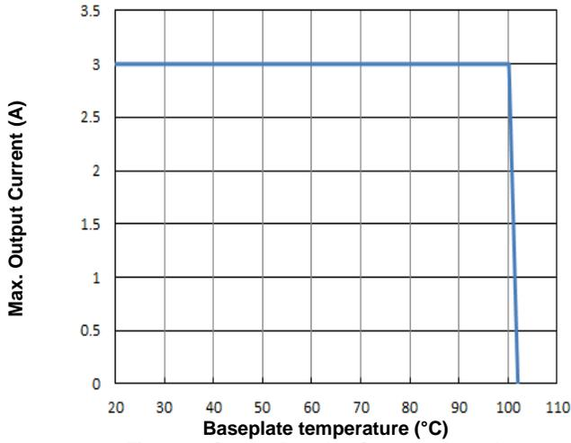
**Figure 9.** Current Derating Curve for Baseplate
