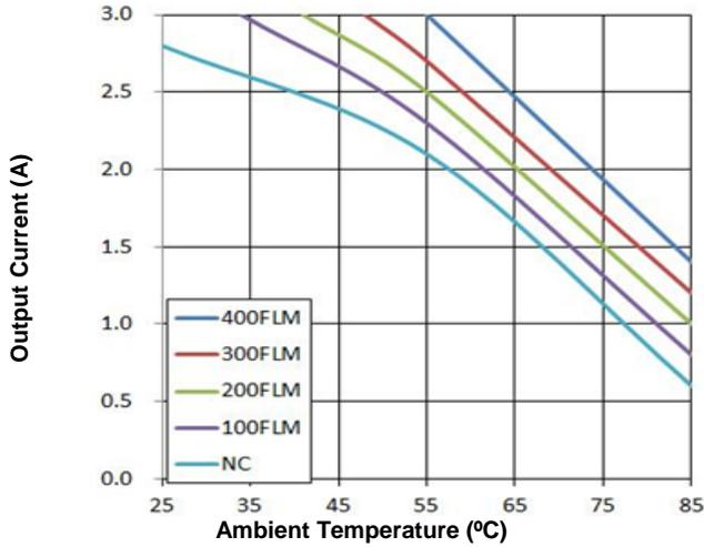
**Figure 7.** Current Derating Curve for Airflow Direction 3
