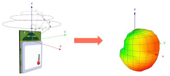
Figure 5: Measurement procedure for radiation patterns
