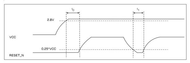
Figure 4: Module power-up and reset timing
