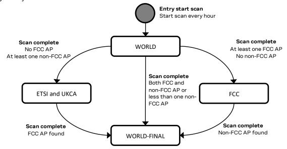
Figure 2: NORA-W2 series IEEE 802.11d state transition diagram
