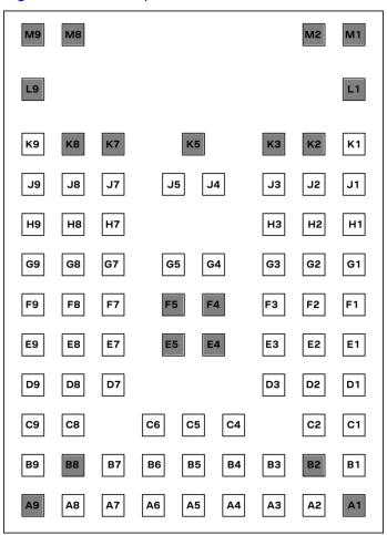
Figure 3: NORA-W251AWS/W256AWS pin assignment (top view)
