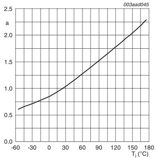
$a = \frac{R_{DSon}}{R_{DSon(25^\circ C)}}$
