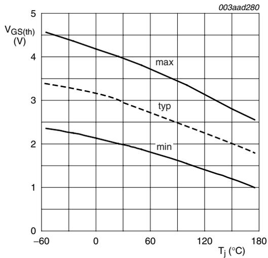
$I_D = 1 mA; V_{DS} = V_{GS}$
