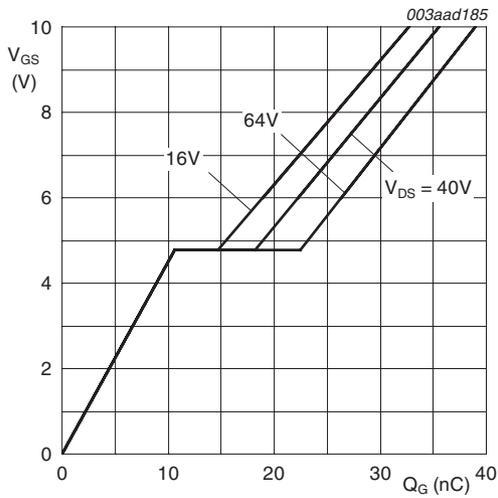
$T_j = 25^\circ\text{C}; I_D = 10\text{A}$
