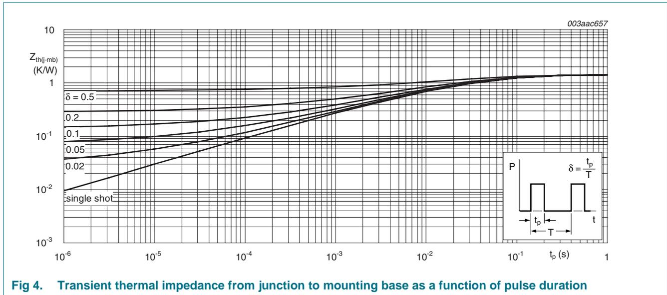
**Fig 4. Transient thermal impedance from junction to mounting base as a function of pulse duration**
