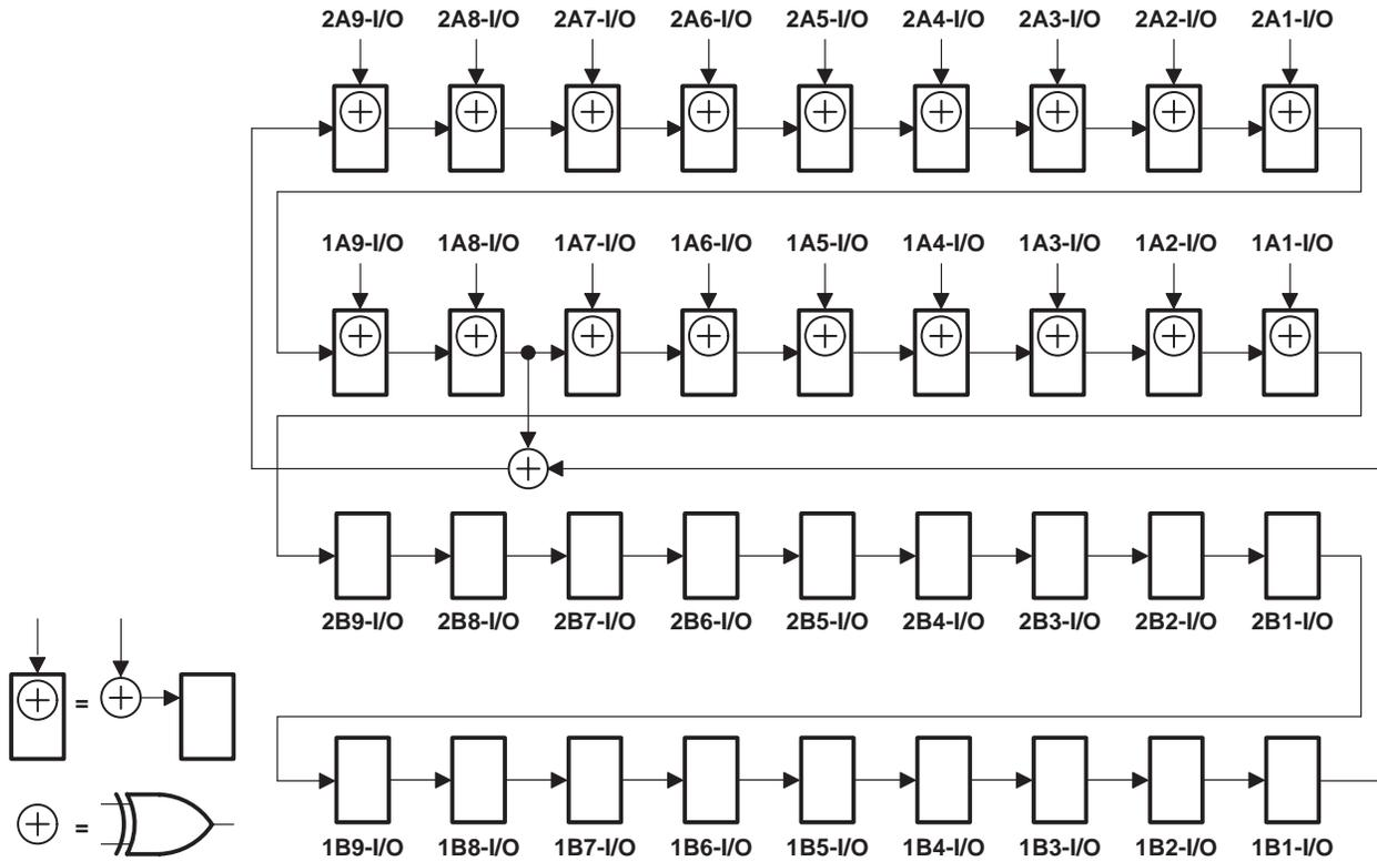
Figure 7. 36-Bit PSA Configuration (10EA = 20EA = 0, 10EB = 20EB = 1)
