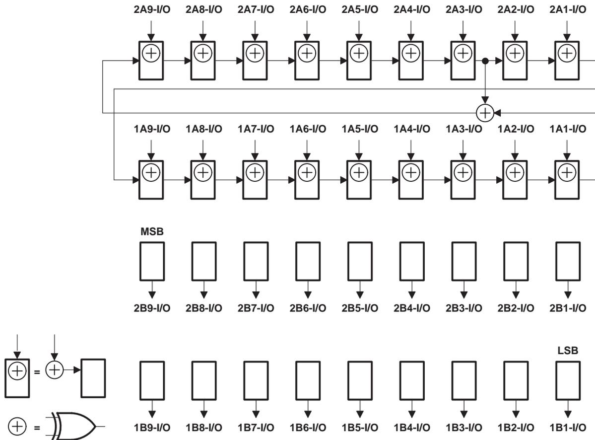
Figure 11. 18-Bit PSA/COUNT Configuration (10EA = 20EA = 0, 10EB = 20EB = 1)
