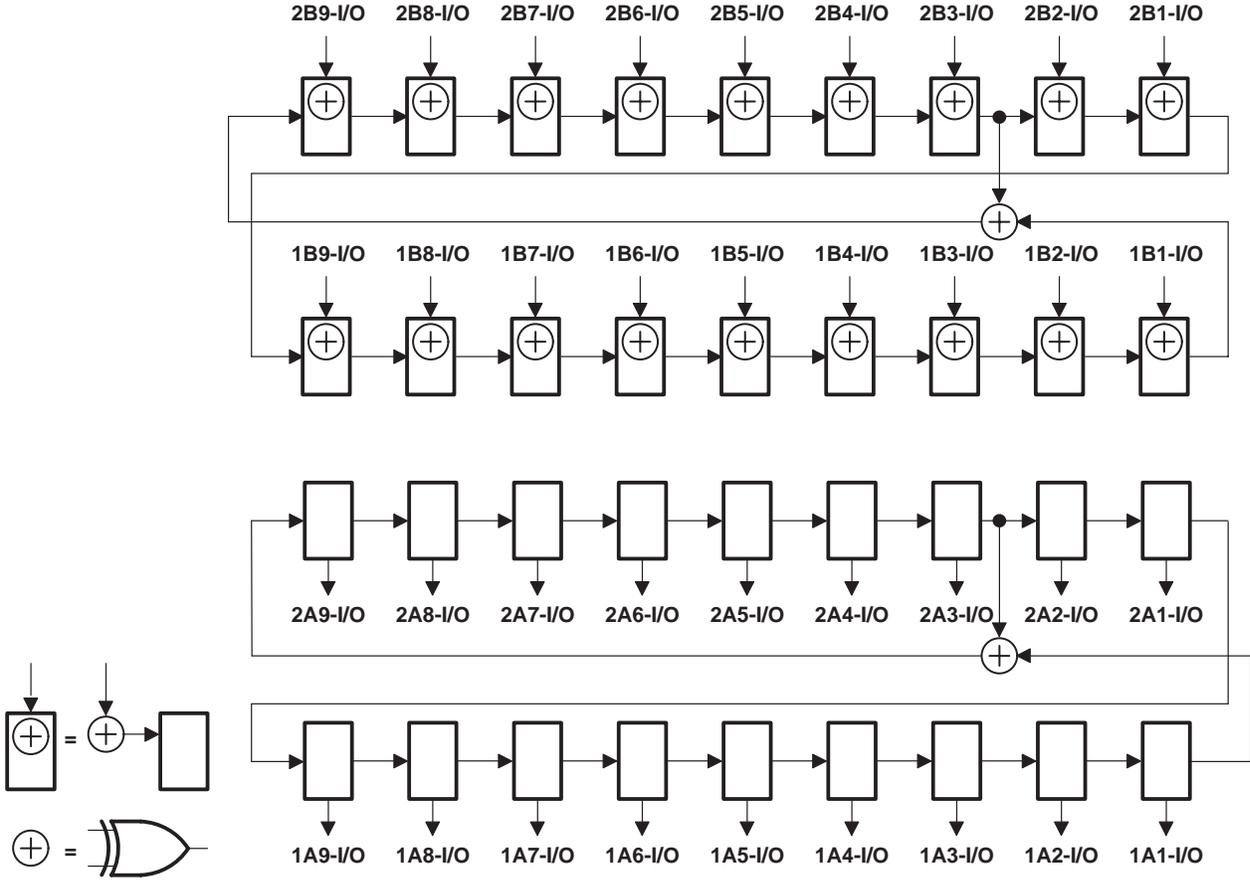
Figure 10. 18-Bit PSA/PRPG Configuration (1OEA = 2OEA = 1, 1OEB = 2OEB = 0)
