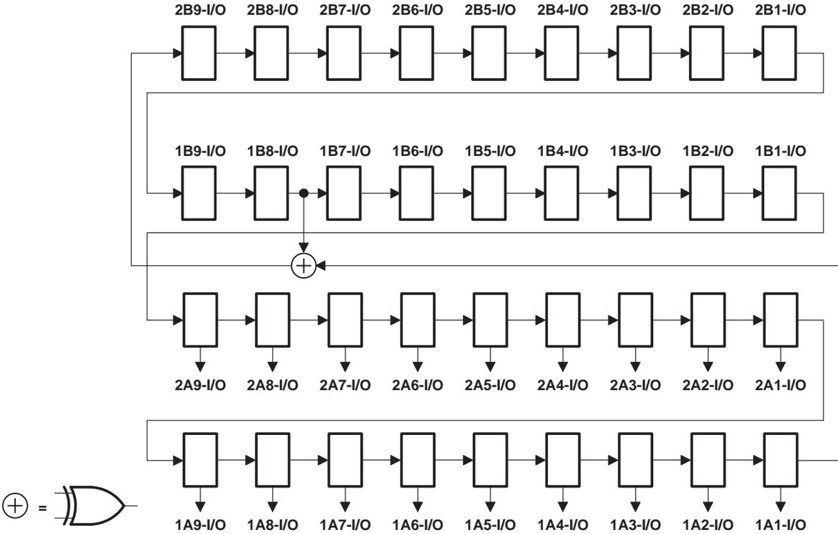
Figure 6. 36-Bit PRPG Configuration (10EA = 20EA = 1, 10EB = 20EB = 0)
