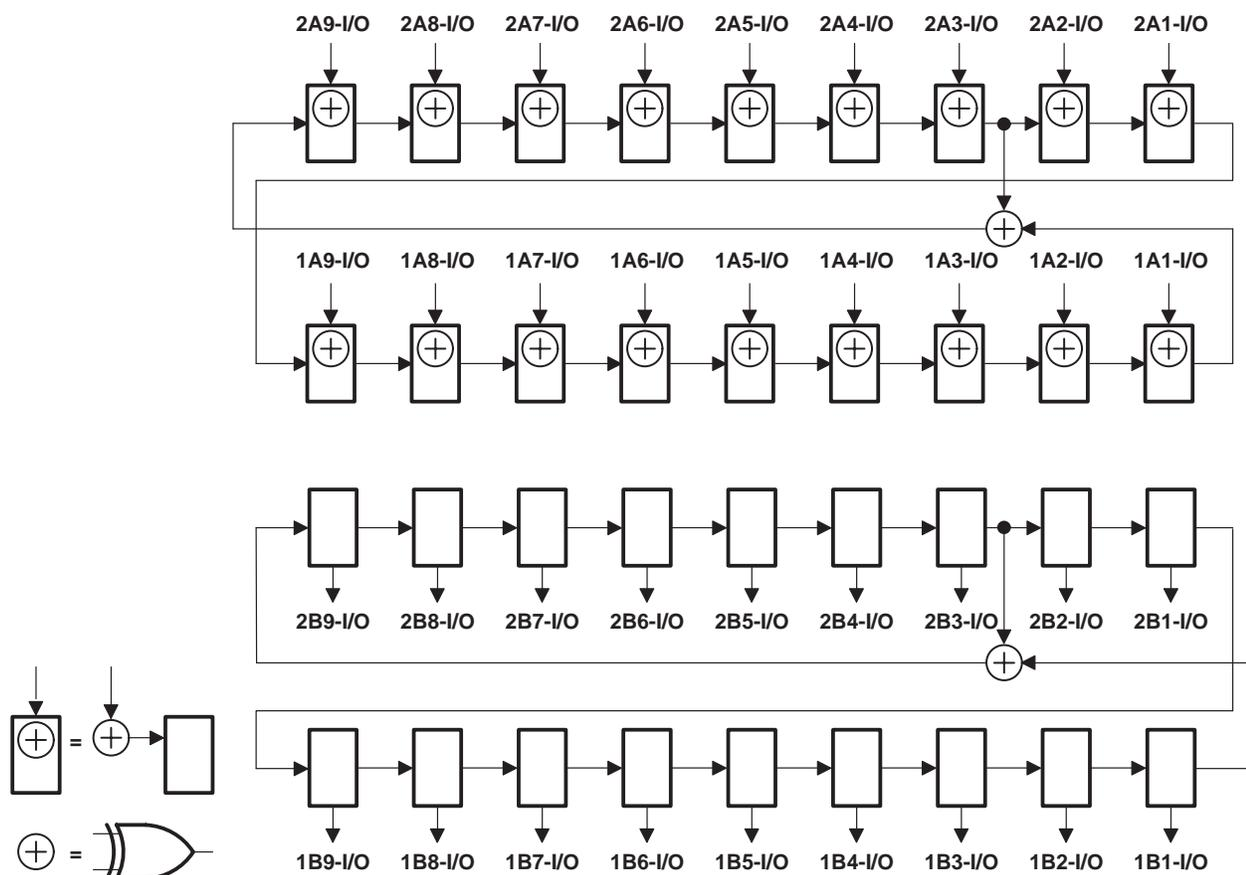
**Figure 9. 18-Bit PSA/PRPG Configuration (10EA = 20EA = 0, 10EB = 20EB = 1)**
