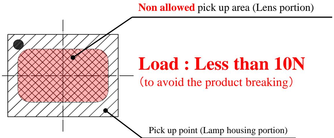
Please adjust the load, the pick up point, the nozzle diameter and etc. before mounting because the over load can cause the breakage of the lamp housing.
