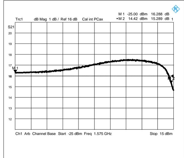
Fig 11. 1dB Gain compression 1.575 GHz 1850 Mhz jammer
