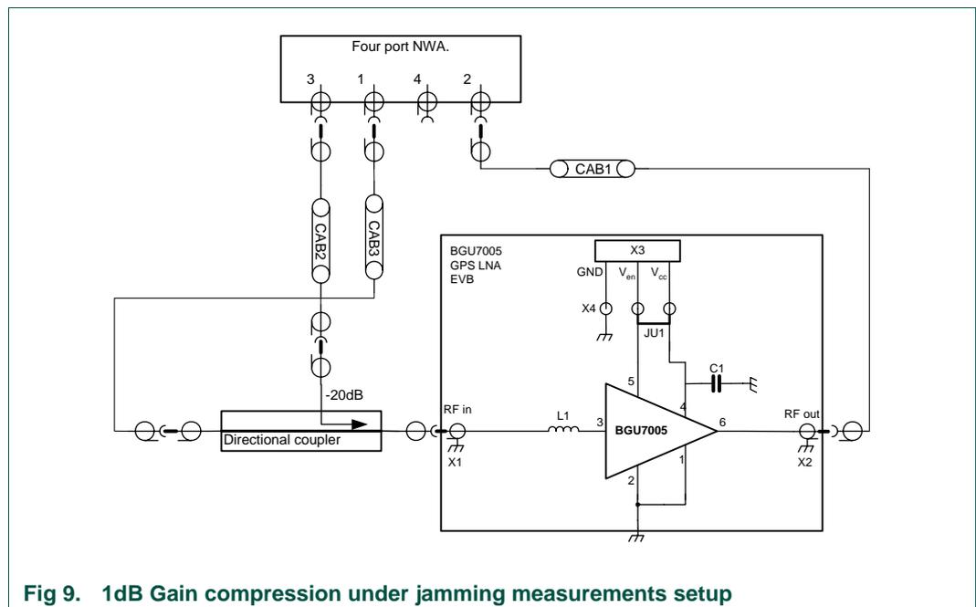
**Fig 9. 1dB Gain compression under jamming measurements setup**
