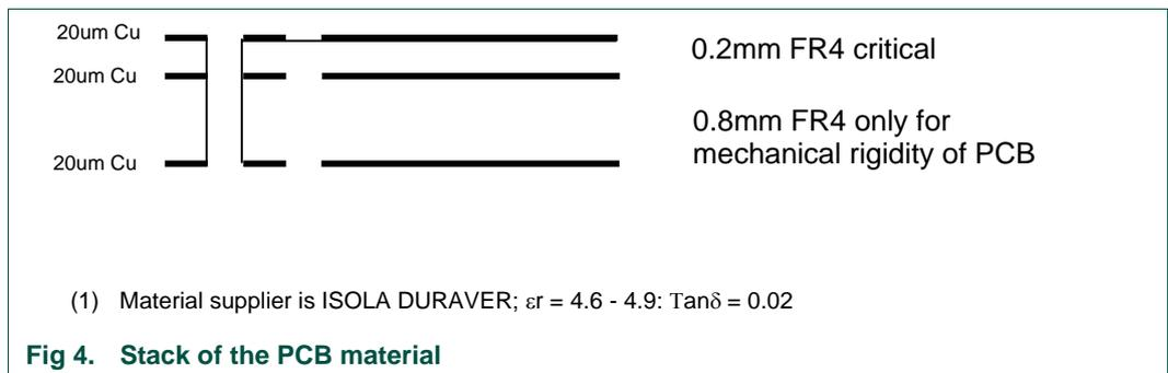
Fig 4. Stack of the PCB material
