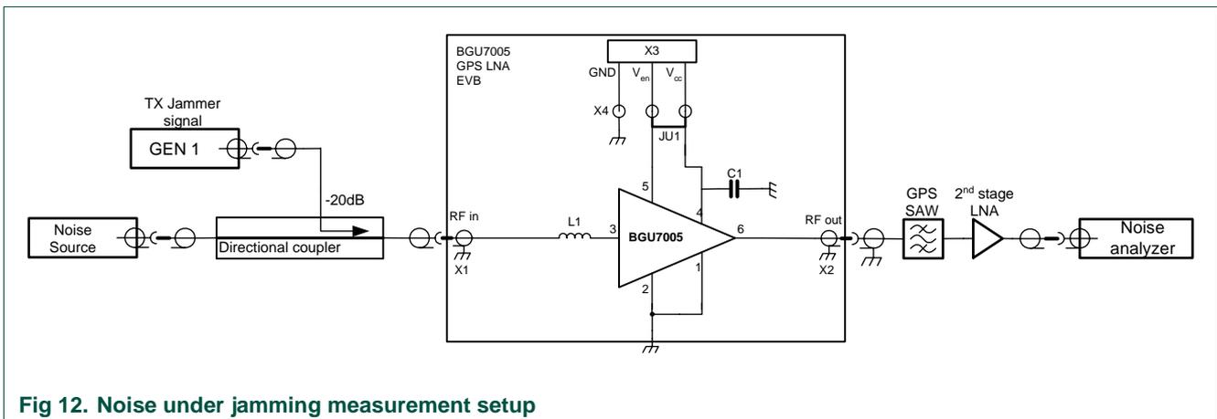
Fig 12. Noise under jamming measurement setup
