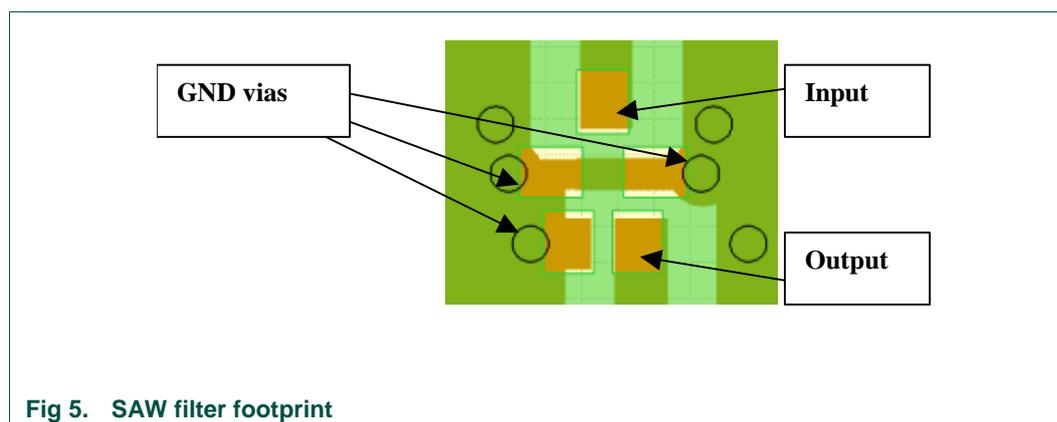
Fig 5. SAW filter footprint
