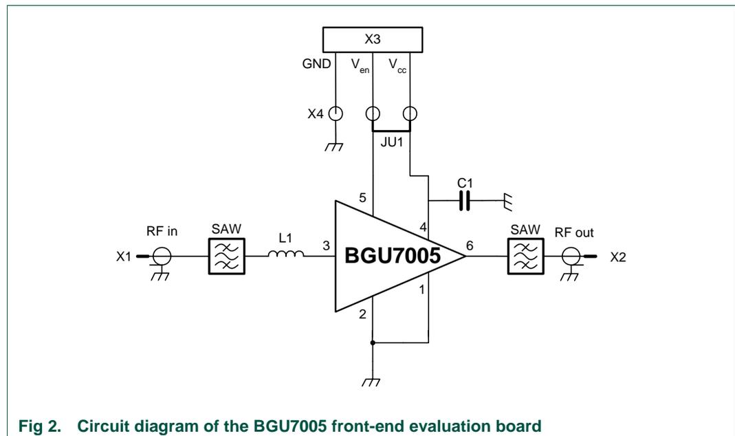
Fig 2. Circuit diagram of the BGU7005 front-end evaluation board
