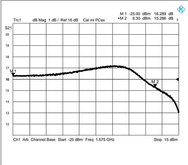
Fig 10. 1dB Gain compression 1.575 GHz 850 Mhz jammer
