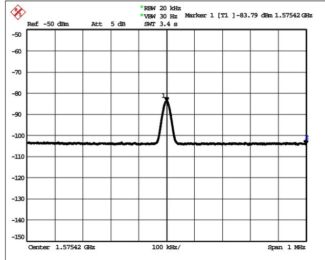
**Fig 8. FE output IM3 level at 1575.42MHz**
