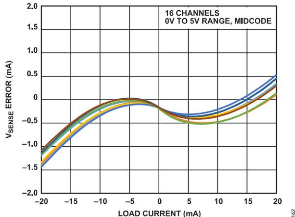
Figure 41.  $V_{SENSE}$  Error vs. Load Current from Equation 5
