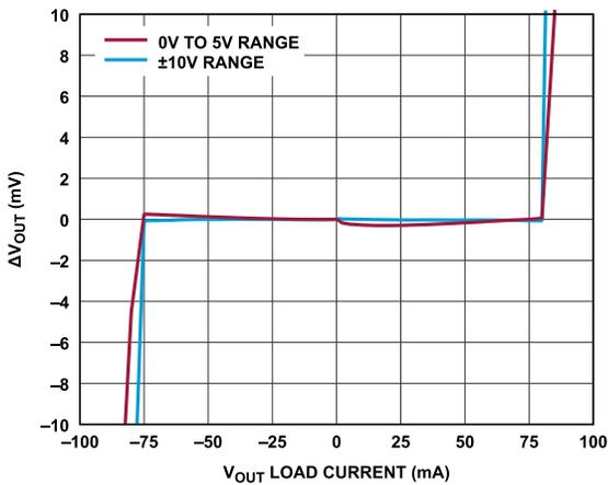
Figure 18.  $\Delta V_{OUT}$  vs.  $V_{OUT}$  Load Current
