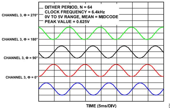
Figure 24. Sinusoidal Dither for Various Phase Settings
