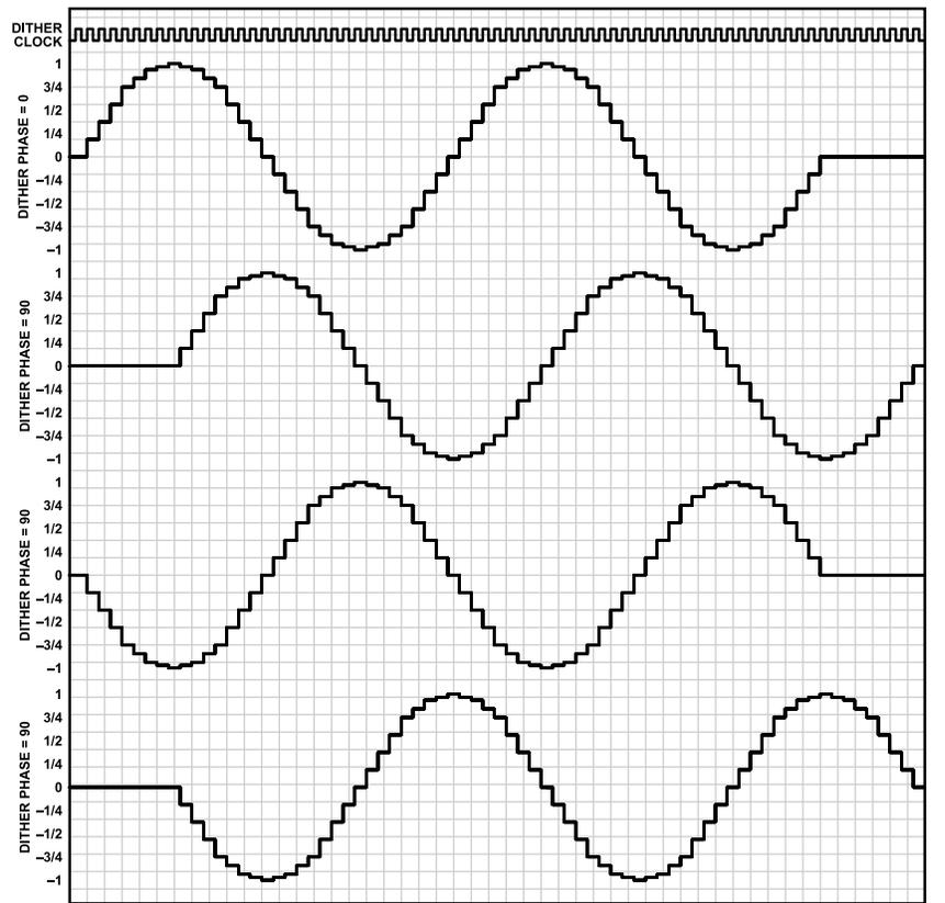
Figure 51. Sinusoidal Waveforms for Various Values of  $\Phi_0$
