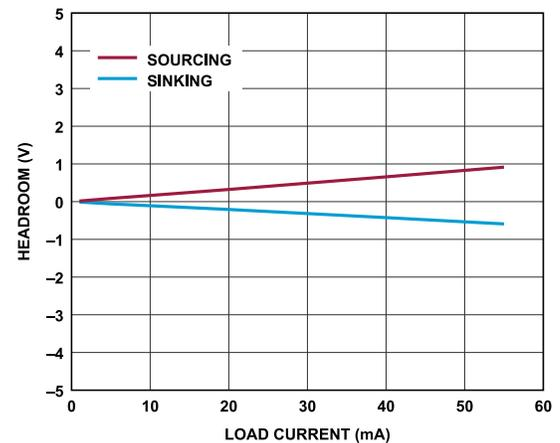
Figure 39.  $V_{x^+}/V^-$  Unipolar Headroom vs. Output Load Current
