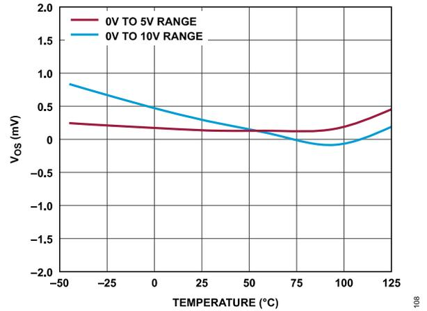
Figure 8. Unipolar Offset Error ( $V_{OS}$ ) vs. Temperature
