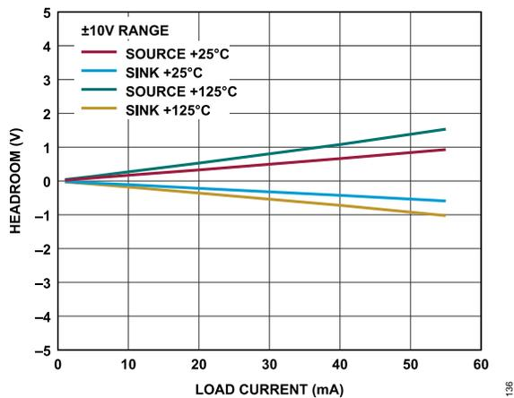
Figure 40.  $V_{x^+}/V^-$  Bipolar Headroom vs. Output Load Current
