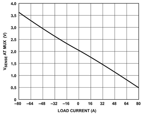
Figure 20.  $V_{SENSE}$  at MUX vs. Load Current
