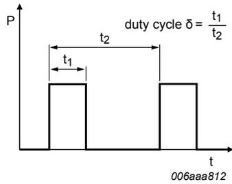
Fig. 17. Duty cycle definition
