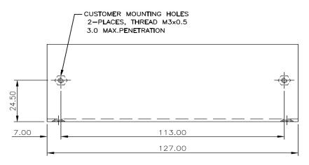
MECHANICAL OUTLINE DIMENSIONS ALL DIMENSIONS ARE IN MM GEN.TOLERANCE:+/-0.5 MM
