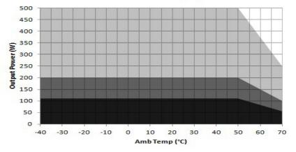
Convection load: 110W up to 50 °C De-rate above 50 °C @ 2.5% per °C
