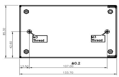
MECHANICAL OUTLINE DIMENSIONS ALL DIMENSIONS ARE IN MM. GEN. TOLERANCE:  $\pm 1.0~\mathrm{mm}$
