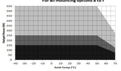
Convection load: 150W UP TO 50 °C De-rate above 50 °C @ 2.5% per °C
