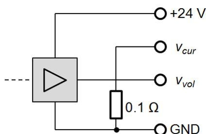
**Fig. 2.** Output stage of the CeraPlas driving circuit
