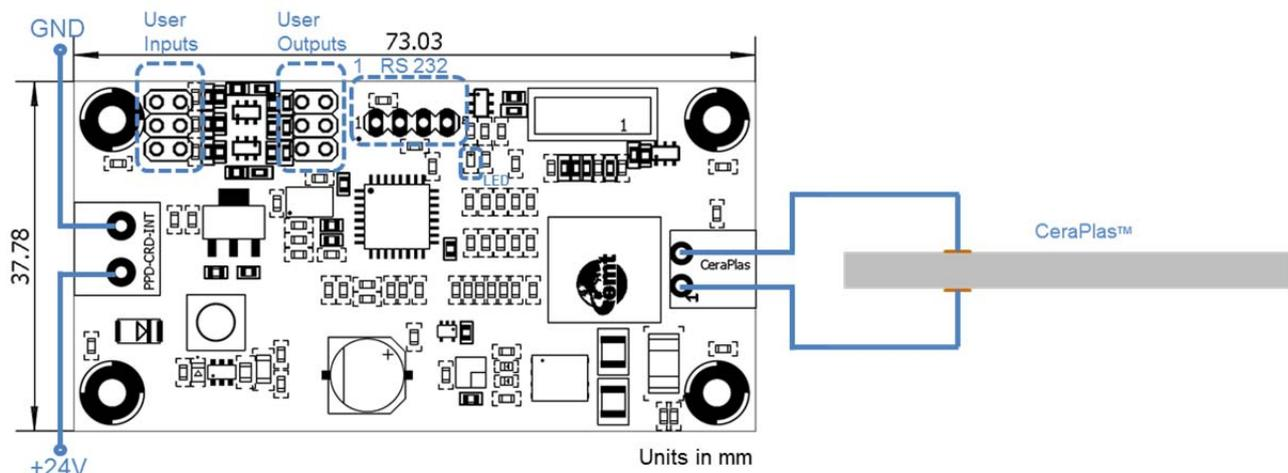
Fig. 1. CeraPlas driving circuit connection setup
