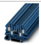
Feed-through terminal block, Connection type: Screw connection, Cross section: 0.14 mm² - 6 mm², AWG: 26 - 10, Nominal current: 20 A, Nominal voltage: 500 V, Length: 65.4 mm, Width: 6.2 mm, Color: blue, Assembly: NS 35/7,5, NS 35/15
