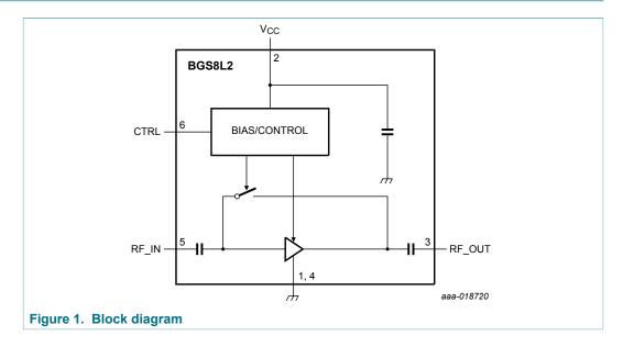
SiGe:C Low-noise amplifier MMIC with bypass switch for LTE
