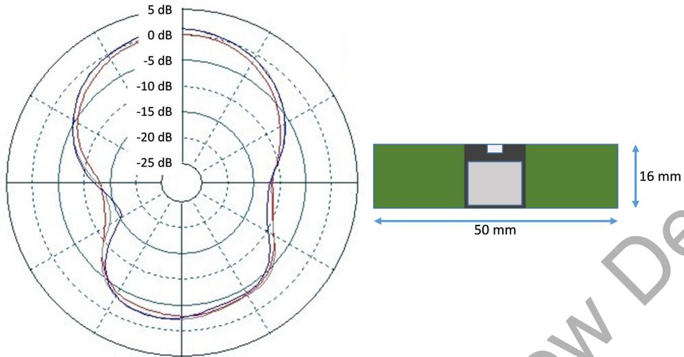
Figure 4.6. Typical 2D Radiation Pattern – Top View
