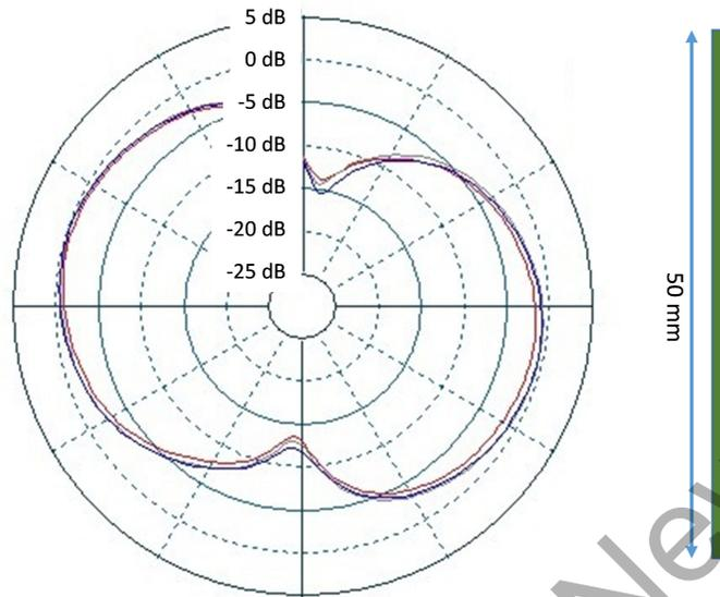
Figure 4.4. Typical 2D Radiation Pattern – Front View
