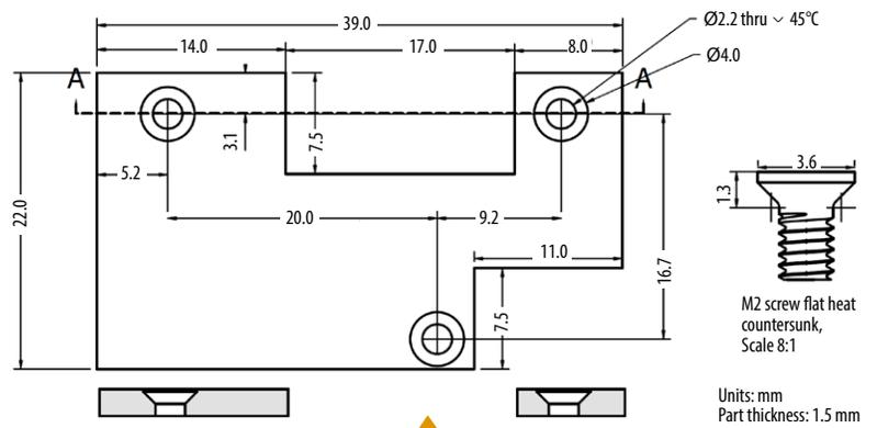
Figure 10: Heat-spreader details
