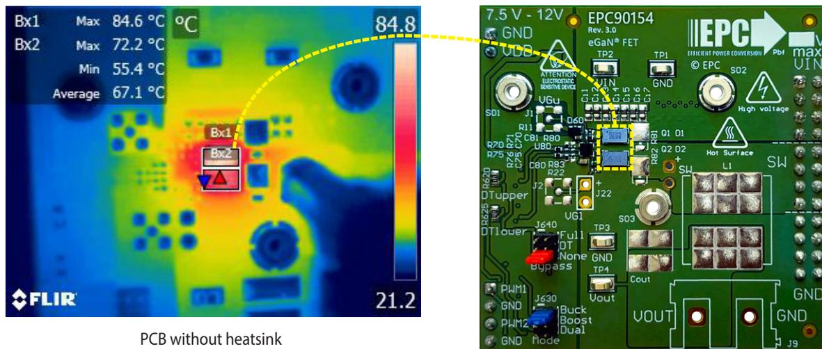
Figure 16: Measured thermal image reading of case temperature when operating under the following conditions:
