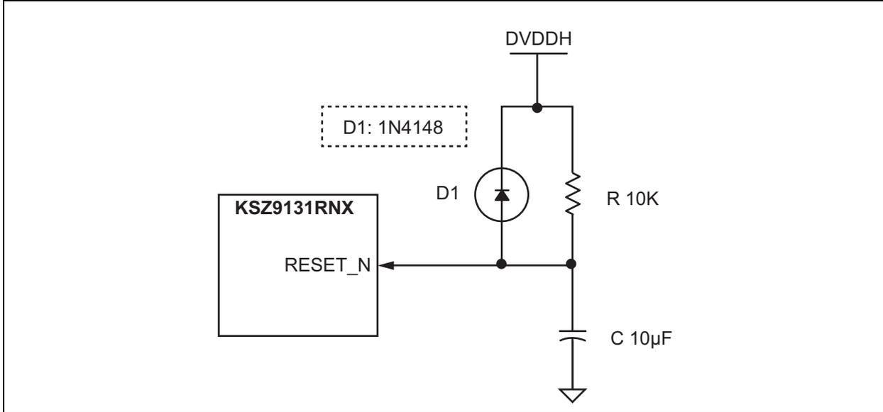
Figure 6-9 illustrates the reset circuit for applications where reset is driven by another device (for example, the CPU or an FPGA). At power-on-reset, R, C, and D1 provide the monotonic rise time to reset the KSZ9131RNX device. The RST\_OUT\_N from the CPU/FPGA provides the warm reset after power-up.
