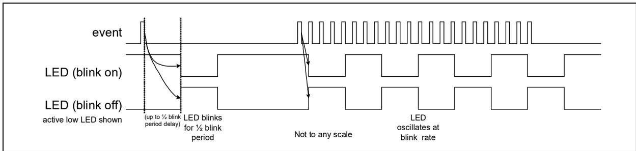
Pulse-stretch ensures that an LED is asserted and de-asserted for a specific period of time when activity is either present or not present.
