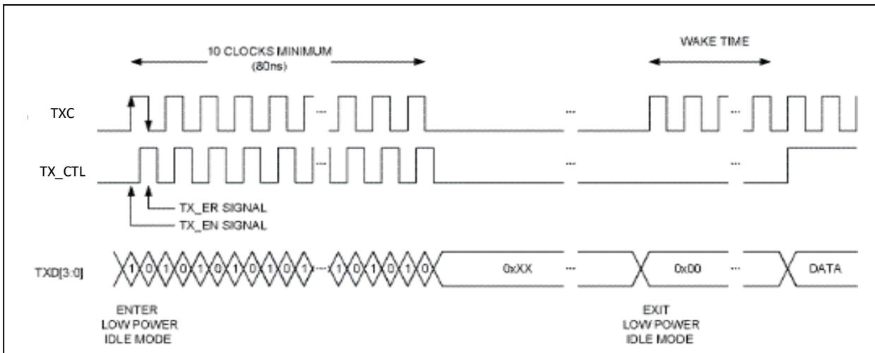
RGMII 100 Mbps transmission from MAC-to-PHY uses both rising and falling edges of the TXC clock. The KSZ9131RNX uses the TX\_CTL pin to clock in the TX\_EN signal on the rising edge and the TX\_ER signal on the falling edge. It also uses the TXD[3:0] pins to clock in the TX data Bits [3:0] on the rising edge.
