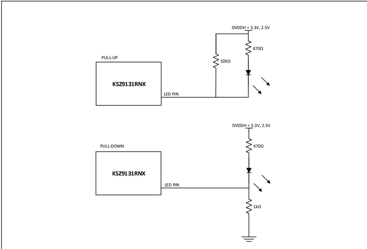
For 1.8V DVDDH, LED indication support requires voltage level shifters between LED[2:1] pins and LED indicator diodes to ensure the multiplexed PHYAD[1:0] strapping pins are latched in high/low correctly. If LED indicator diodes are not implemented, the PHYAD[1:0] strapping pins just need 10 kΩ pull-up to 1.8V DVDDH for a value of 1, and 1.0 kΩ pull-down to ground for a value of 0.
