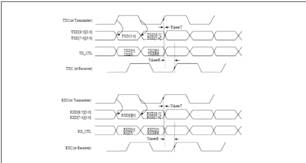
**FIGURE 4-7: RGMII V2.0 SPEC (MULTIPLEXING AND TIMING DIAGRAM - ORIGINAL RGMII (V2.0) WITH INTERNAL DELAY**
