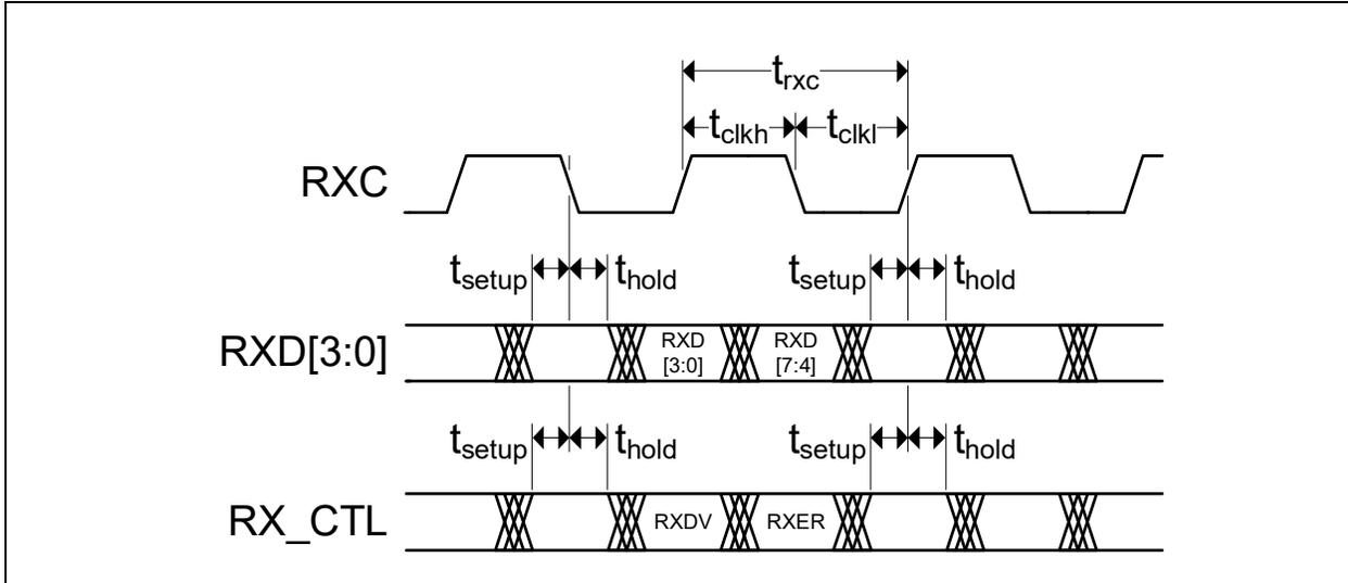
**TABLE 6-14: RGMII RXC INTERNAL DELAY ENABLED (RGMII ID MODE) TIMING VALUES**
