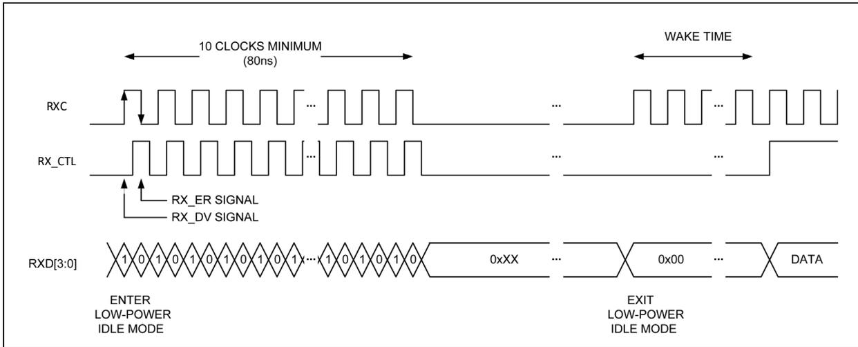
RGMII 100 Mbps reception from PHY-to-MAC uses both rising and falling edges of the RXC clock. The KSZ9131RNX uses the RX\_CTL pin to clock out the RX\_DV signal on the rising edge and the RX\_ER signal on the falling edge. It also uses the RXD[3:0] pins to clock out the RX data Bits [3:0] on the rising edge.
