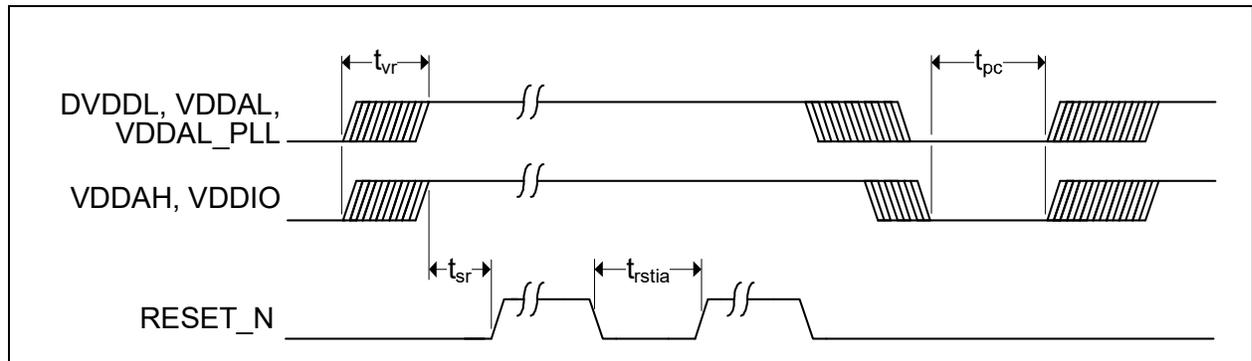
The recommended power-up sequence is to have the transceiver (AVDDH) and digital I/O (DVDDH) voltages power up before the 1.2V core (DVDDL, AVDDL, AVDDL\_PLL) voltage. If the 1.2V core must power up first, the maximum lead time for the 1.2V core voltage with respect to the transceiver and digital I/O voltages should be 200  $\mu$ s.
